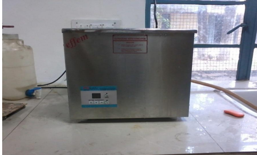
Fig. 4.4: Sonication being done for evenly dispersing nanoparticles
