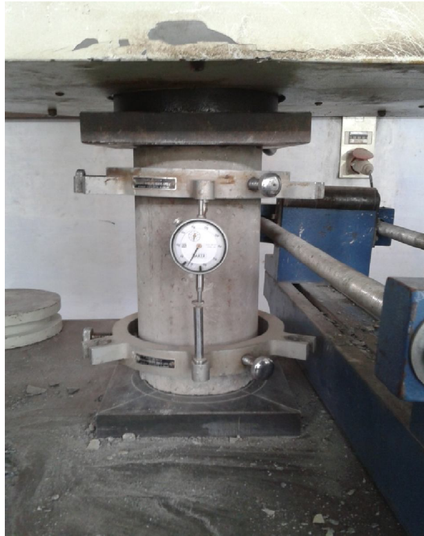
Fig. 3.3 Setup for Young's Modulus using Extensometer
