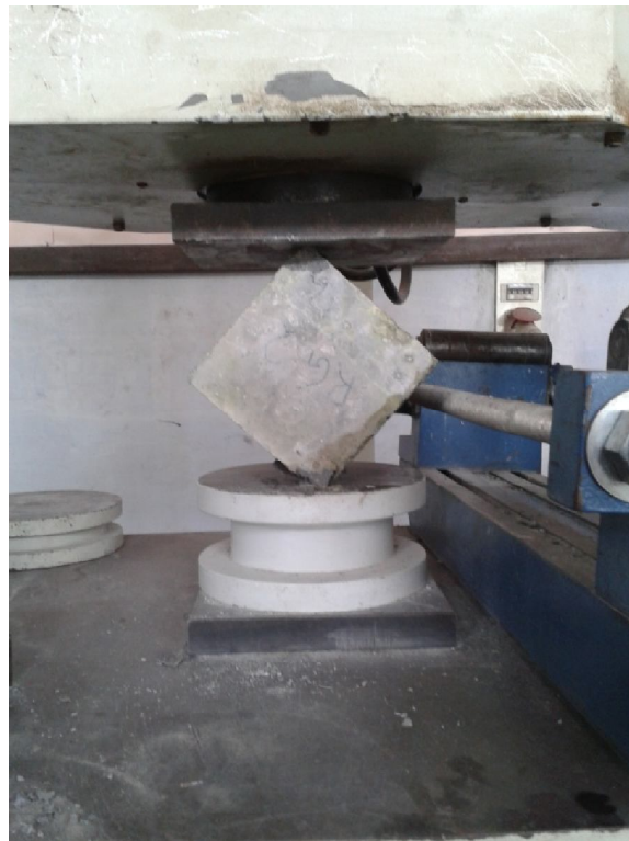
Fig. 3.2 Setup for Split Tensile Strength
