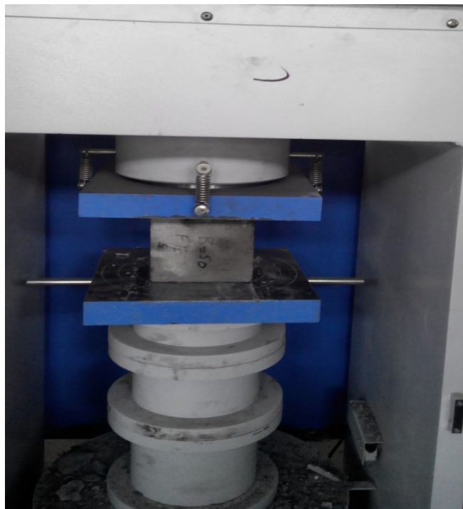
Fig. 3.1 Setup for Compressive Strength
