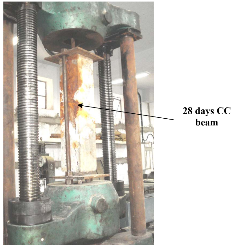
Fig. 5.18: Beam undergoing pull out test in a UTM
