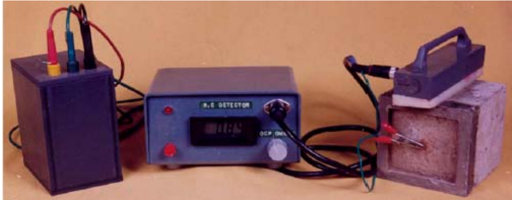
Fig 3.15: Galvanostatic pulse instrument with probe and concrete sample (Sathiyarayanan et al., 2006)
