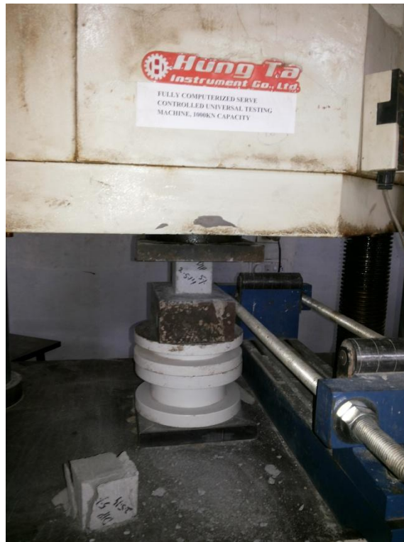
Fig. 3.5: Compressive Strength Testing of Cube under UTM
