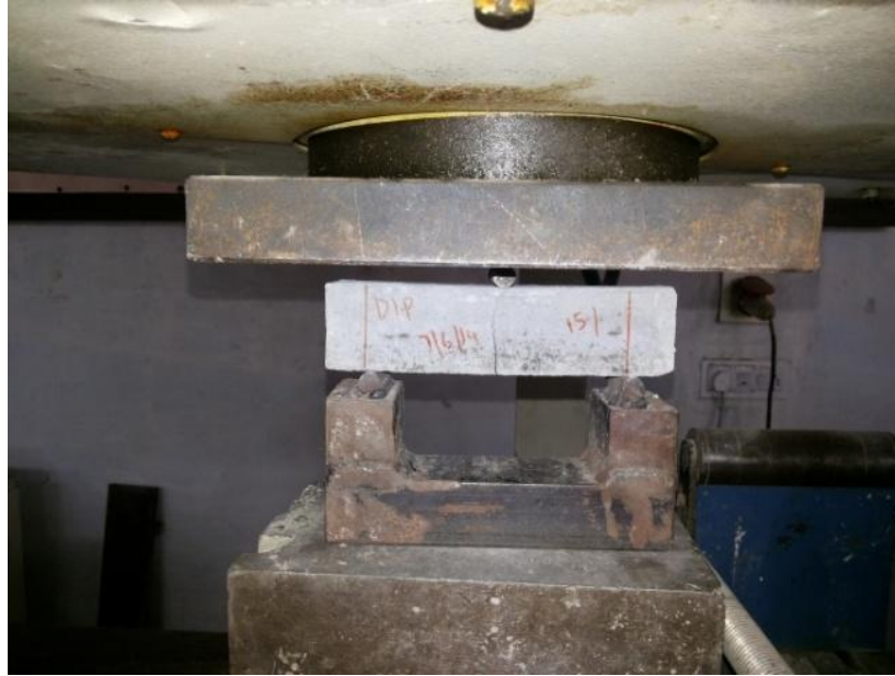
Fig. 3.7: Flexural Strength Testing of Specimen under UTM by Three Point Loading
