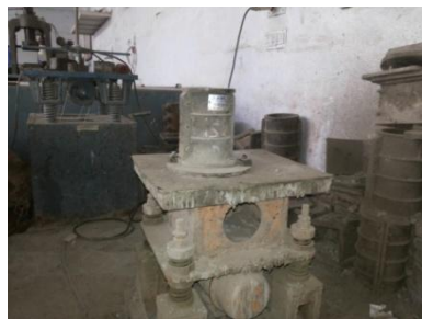
Fig. 3.9 (a) Cylindrical Mould for Specimens of Size 100 mm x 200 mm
