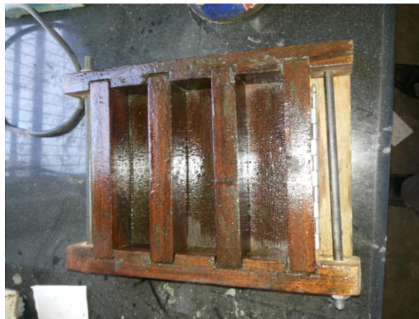
Fig. 3.6: Mould Specimens of Size 40 mm x 40 mm x 160 mm
