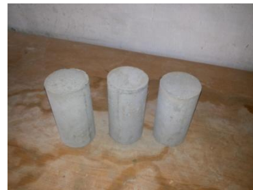
Fig. 3.9 (b) Casted Cylindrical Specimens of Size 100 mm x 200 mm
