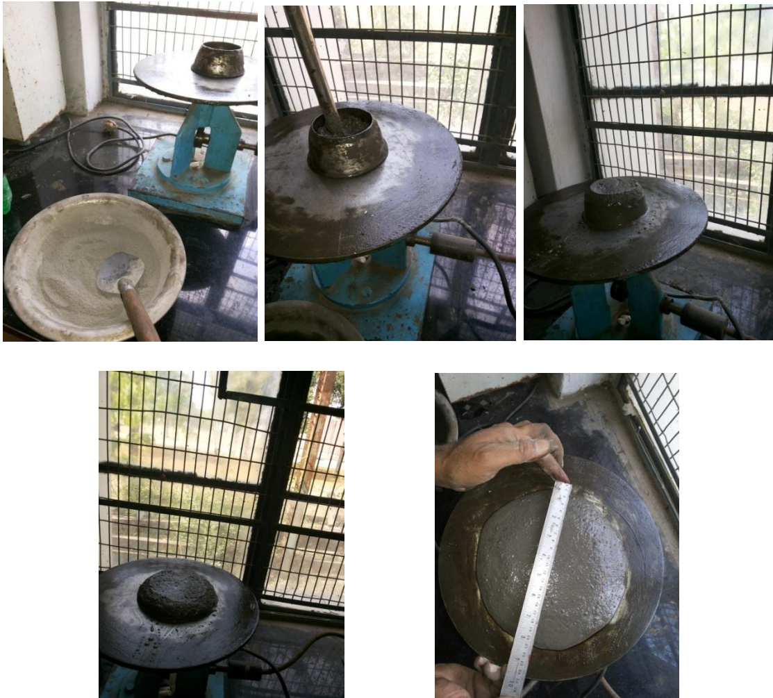
Fig.3.2 Measurement of flow value by Flow Test
