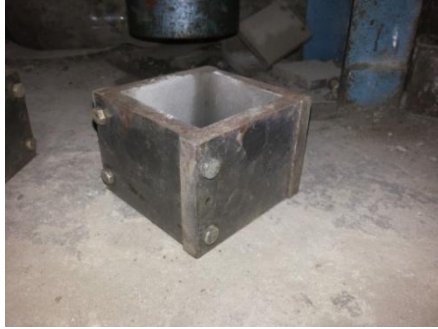
Fig. 3.3: Cube Specimens of Size 70.6 mm x 70.6 mm x 70.6 mm
