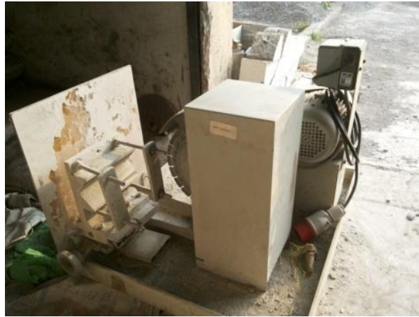
Fig. 3.10: Cylindrical Specimens Cutter Machine
