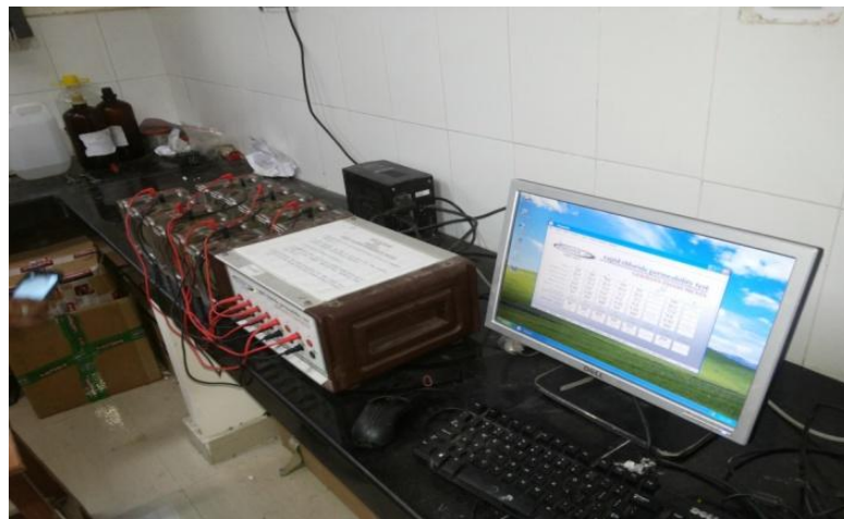
Fig.3.13: Rapid Chloride Permeability Test Setup
