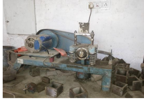
Fig.3.4: Vibrating Machine each Sample to be Vibrated at 12000 Cycles per Minute
