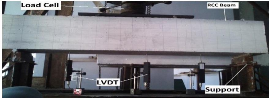
Fig. 3.1(b) Two-point loading setup of RC beam
