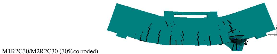
Fig. 4.7(b). Failure patterns of RC beams after FE analysis (shear failure observed)
