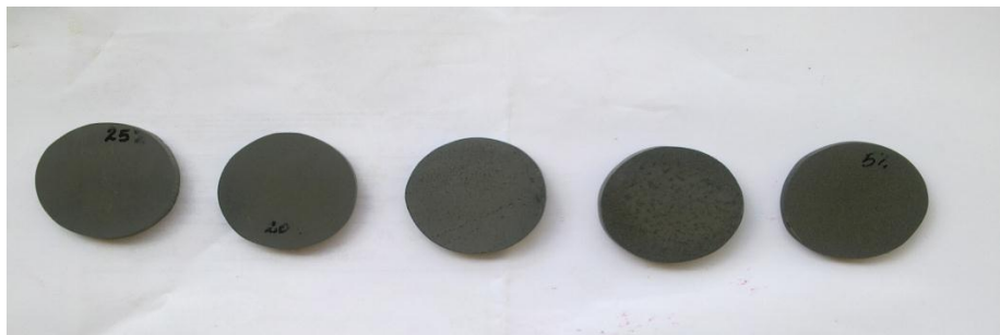
Images of Thermal Conductivity specimens of polyester Al powder composites.
