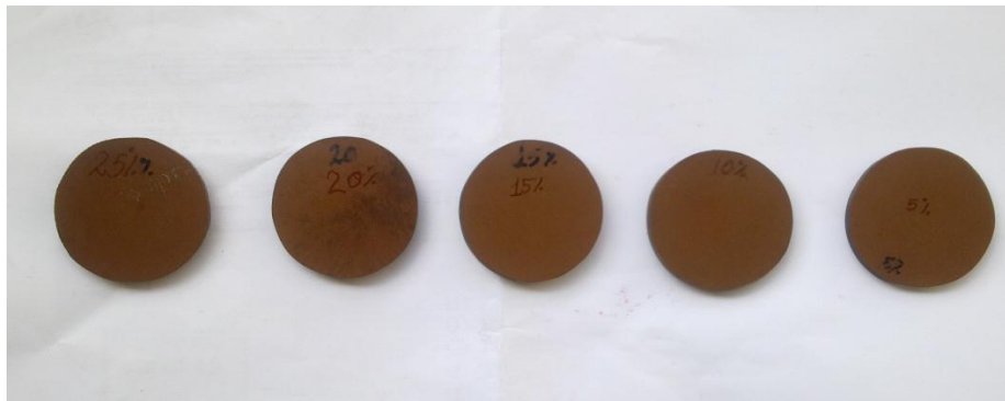
Images of Thermal Conductivity specimens of polyester Cu powder composites.
