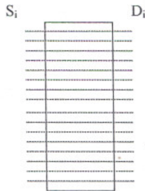
Fig. 3.1: Identity permutation layout for network of size N=16
