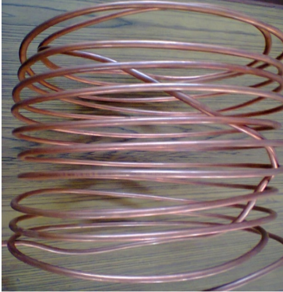
Figure 3.8 – Evaporator coil and evaporator container with water
