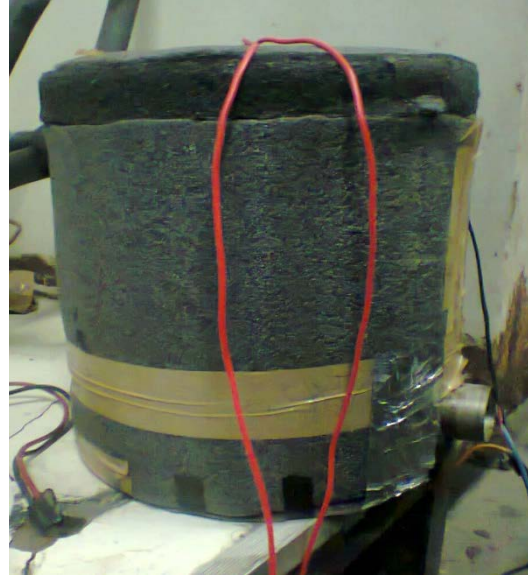
Figure 3.8 – Evaporator coil and evaporator container with water
