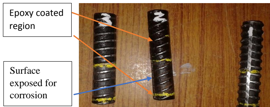
Fig. 3.12. Epoxy coated steel bars used in Stage-III
