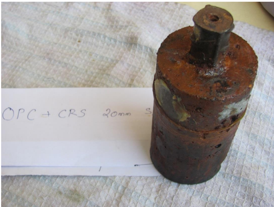
Fig. C-5. Condition of specimen at the end of testing
