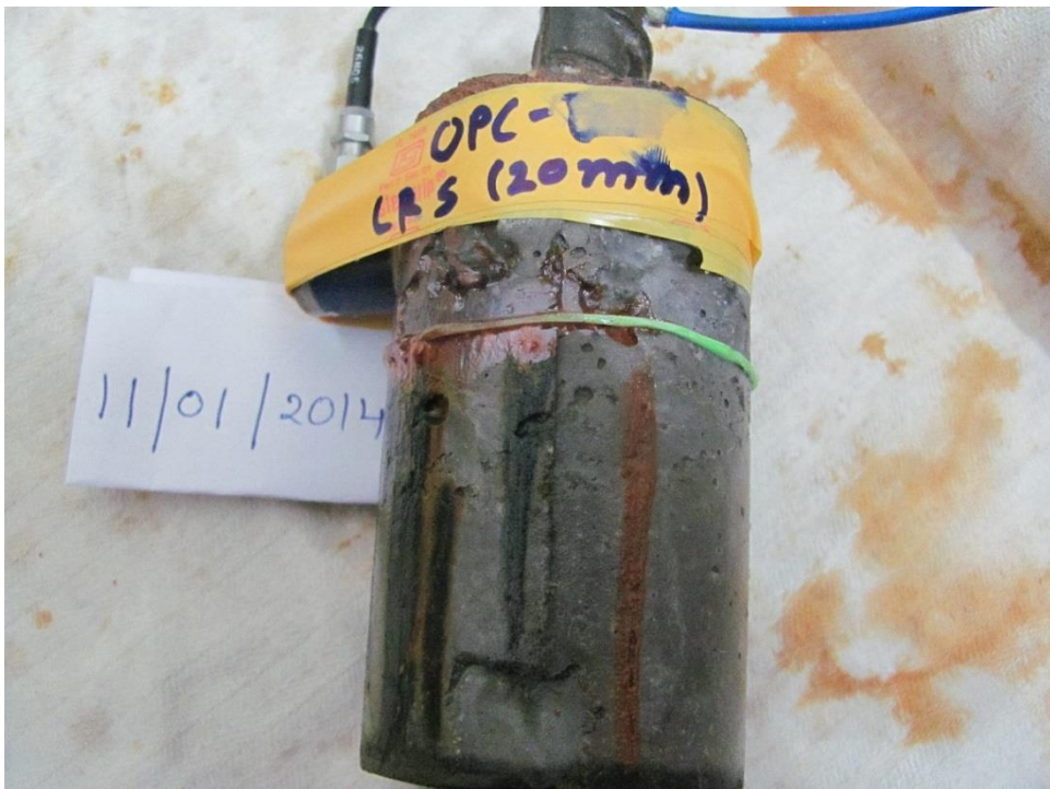
Fig. C-3. Condition of specimen after 4 days of testing
