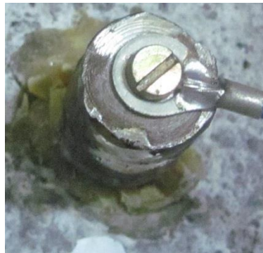
Fig. 3.2. Threaded end of steel rebar with screw for electrical connection
