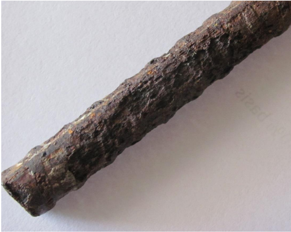
Fig. 6.9. Condition of steel surface after testing using impressed current technique
