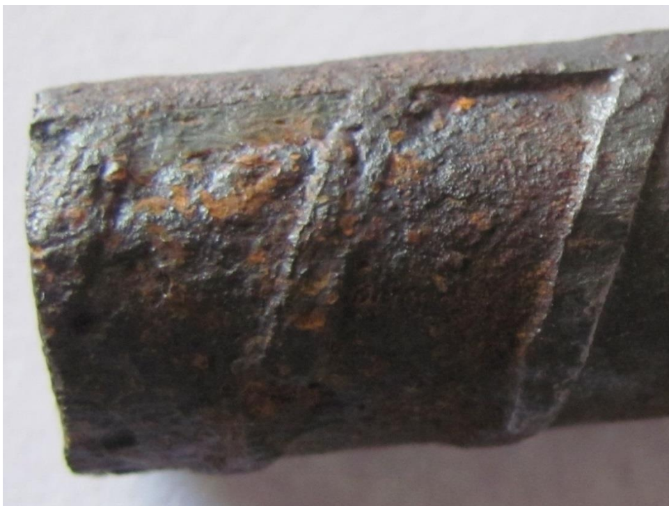
Fig. 6.8. Condition of steel surface after testing using alternate drying-wetting cycles
