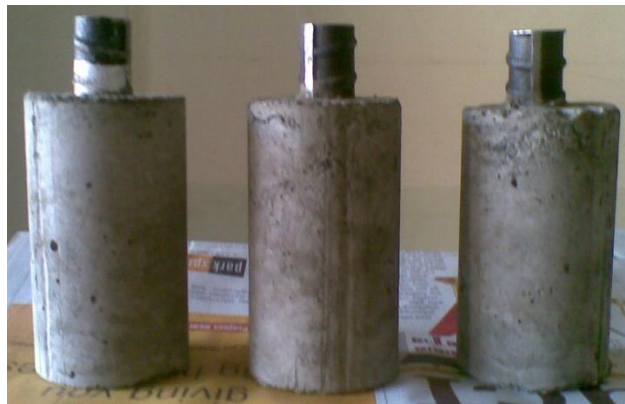
Figure 3.14. Specimens after casting
