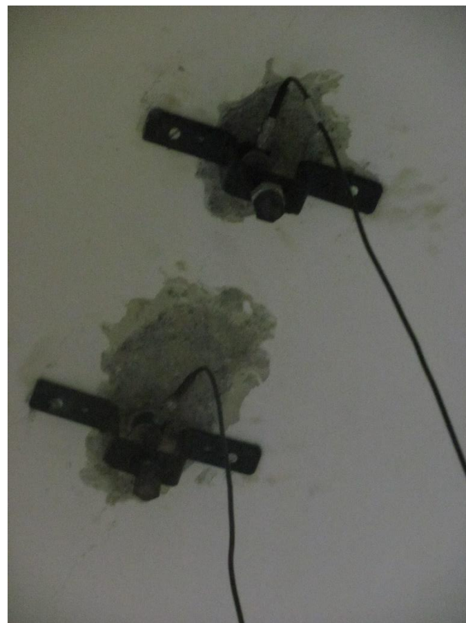
Fig.D-6. Sensors attached to the slab surface using holders
