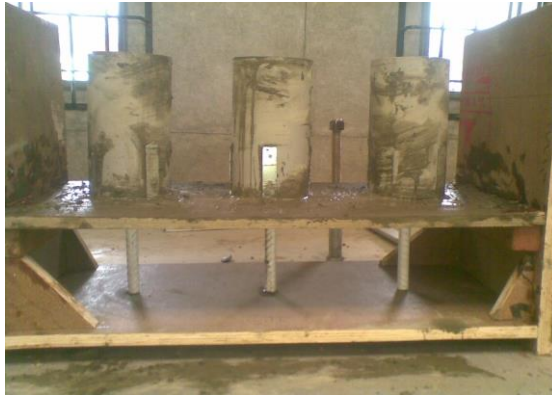
Fig. 3.9. Special molding system used for casting in Stage-II
