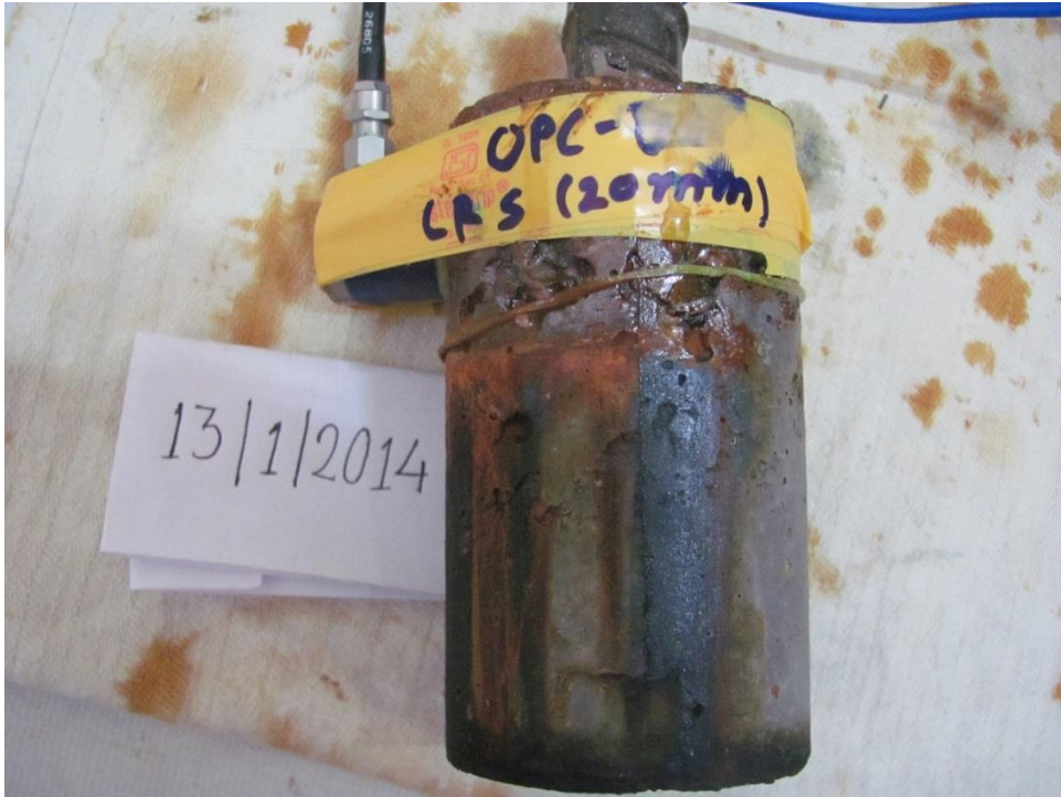
Fig. C-4. Condition of specimen after 6 days of testing
