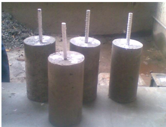
Fig. 3.4. Specimens after casting
