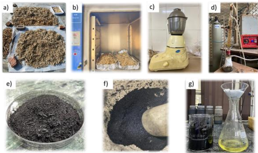
Figure 3.1: a) Sugarcane bagasse being dried in sunlight. b) Sugarcane bagasse being Vacuum oven dried at 70°C. c) Grinding of oven-dried sugarcane bagasse. d) Pyrolysis equipment setup. e) Resultant black powder obtained after Pyrolysis. f) Ground Resultant black powder. g) Washing and Filtering of Resultant black powder.
