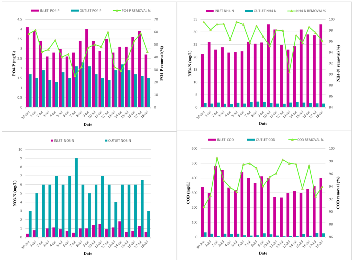
Figure 4.5: Performance Assessment of 3MLD SBR in terms of COD, NH 4 -N, NO 3 -N and PO 4 -P removal
