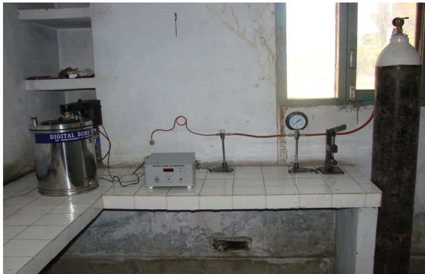
Fig 5.7: Bomb Calorimeter used for measurement of Calorific value
