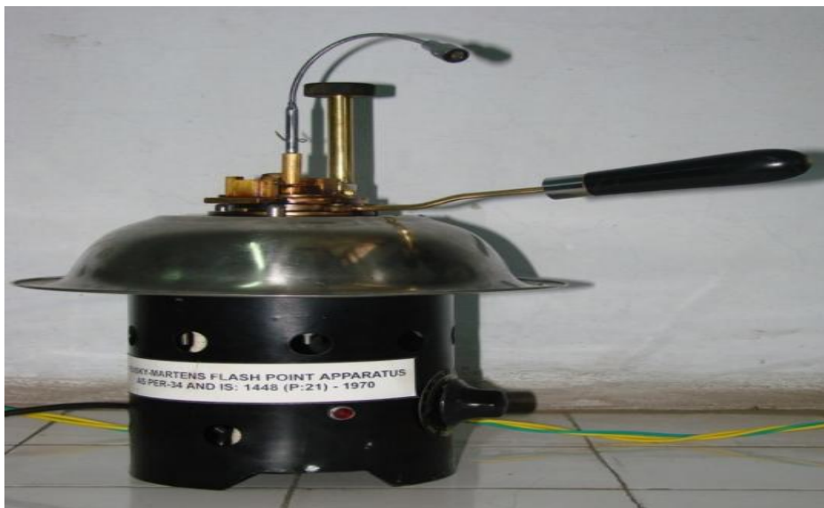
Fig 5.2: Pensky Marten apparatus used for measurement of flash and fire point
