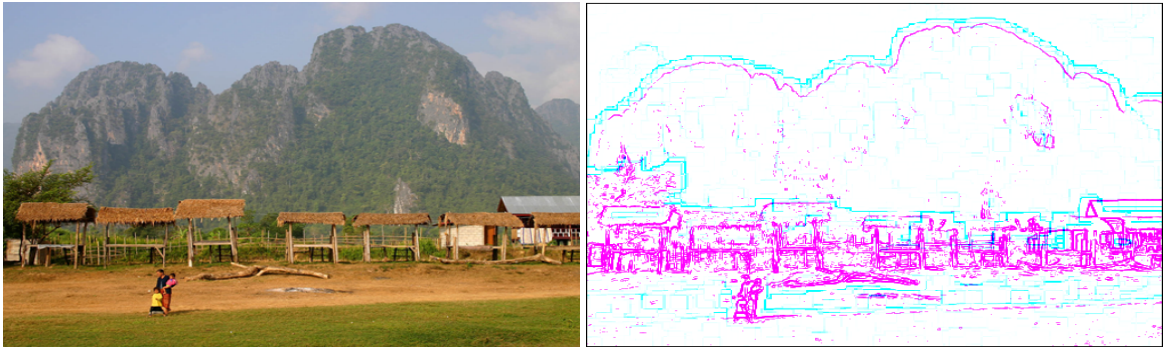
Figure 3.7: Example showing the difference between the original and proposed dark channel with respect to edges
