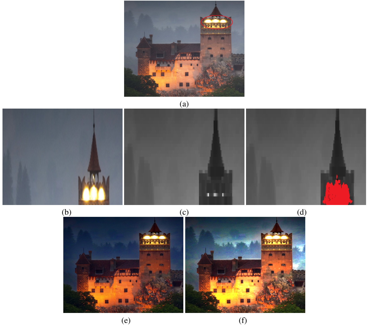
Figure 3.10: Effect of pixels filtering on atmospheric light and overall de-fogged image. (a) Input Image. (b) Top \frac{1}{4} rows of an input image. (c) 15 \times 15 dark channel of image in (b). (d) Bright pixels filtered from (c). (e) Restored image by using dark channel in (c). (f) Restored image by filtering bright pixels in dark channel.
