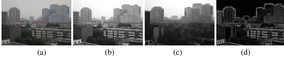
Figure 5.7: (a) Input images. (b) Minimum color channel (c) Dark Channel (d) Difference between minimum color channel and dark channel.
