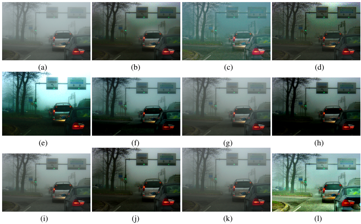
Figure 4.10: De-fogging results (a)Input foggy images “ Foggy_road1 ”. De-fogging results of (b) He et al. (c) Tarel et al. (d) Meng et al. (e)Shiau et al. (f) Choi et al. (g) Zhu et al. (h) Cai et al. (i) Ren et al. (j) Liu et al. (k) Colores et al. (l) Proposed
