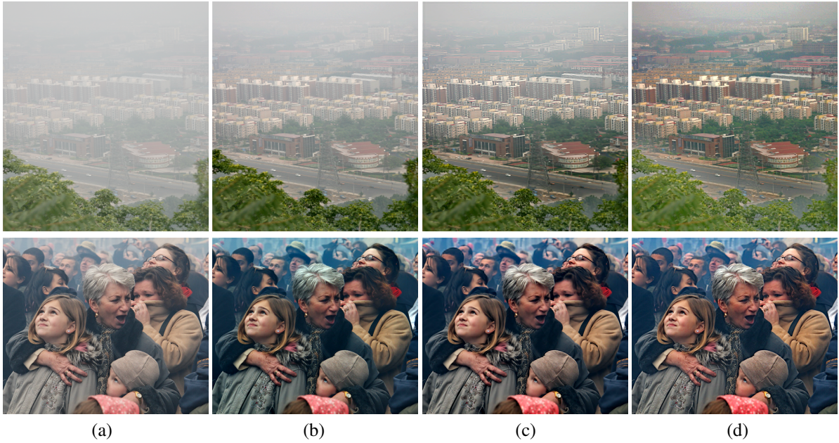
Figure 3.18: De-fogging Results (a) Input foggy images “Cityscape” (top) and “People” (bottom). De-fogging results of (b) Ren et al. (c) Liu et al. (d) Proposed Technique.
