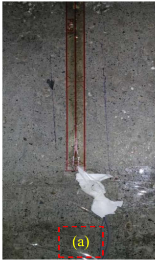
Fig.3. 9 (a) PL-90-11 conventional sensor mounted on concrete beam (b) optical strain gage mounted on steel plate which is then pasted on concrete beam using white cement
