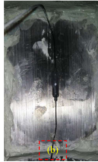
Fig.3. 9 (a) PL-90-11 conventional sensor mounted on concrete beam (b) optical strain gage mounted on steel plate which is then pasted on concrete beam using white cement
