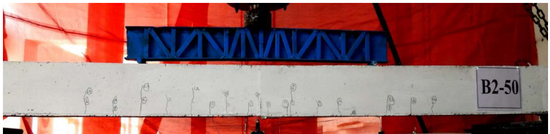
Fig.4. 3 Crack patterns of beam B2-50 when specimen was loaded upto 5kN.
