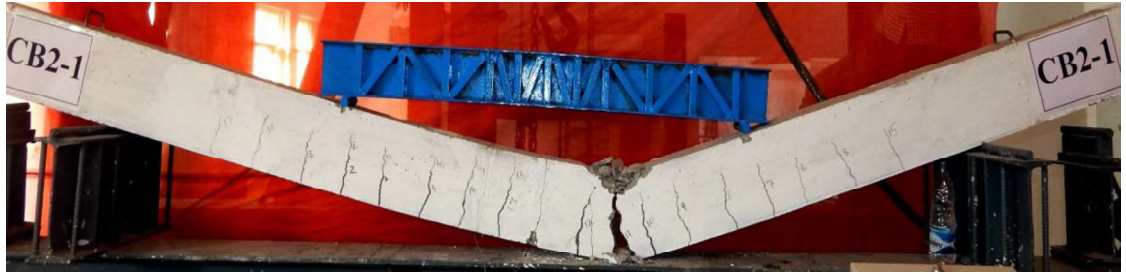
Fig.4. 1 Crack patterns of beam CB2-1 when total failure of specimen occurred.
