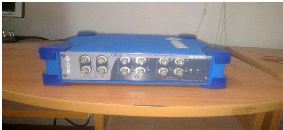
Fig.3. 6 Anlyser that collects all the responses from hammer and accelerometers and provide the FRF
