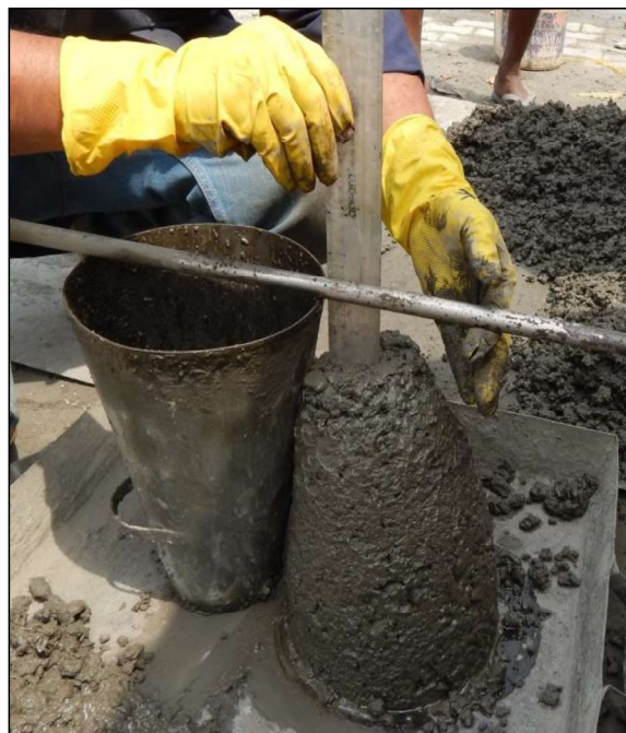
Fig.3. 2 Slump test of green concrete
