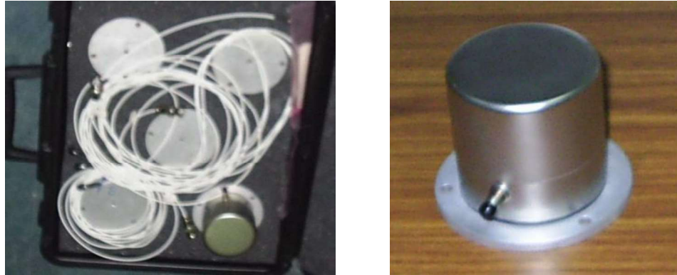
Fig.3. 5 Accelerometers used in vibration monitoring
