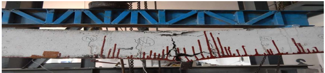
Fig.4. 7 Crack patterns of beam B2-50S when total failure of specimen occurred.
