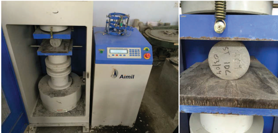
Fig3.7 Cylindrical test specimen tested under UTM
