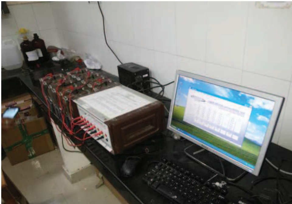
Fig.3.12: Rapid chloride permeability test setup
