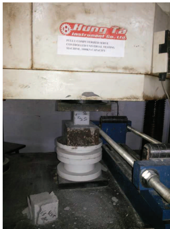
Fig. 3.5: Compressive strength testing of cube under UTM
