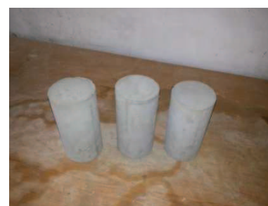
Fig. 3.8 (b) Casted cylinders
