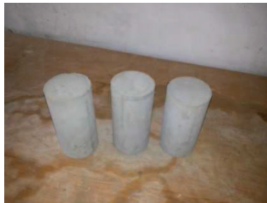
Fig.3.6(b) Casted cylinders
