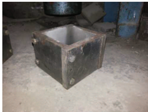
Fig. 3.3: Cube specimens of size 70.6 mm x 70.6 mm x 70.6 mm each sample to be vibrated at 12000 cycles per minute
