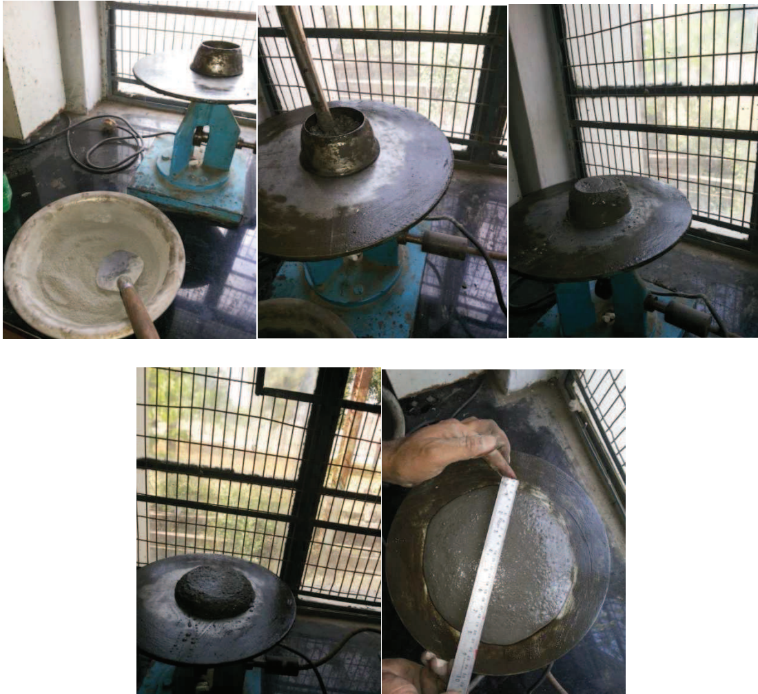
Fig.3.2 Measurement of flow value by flow test
