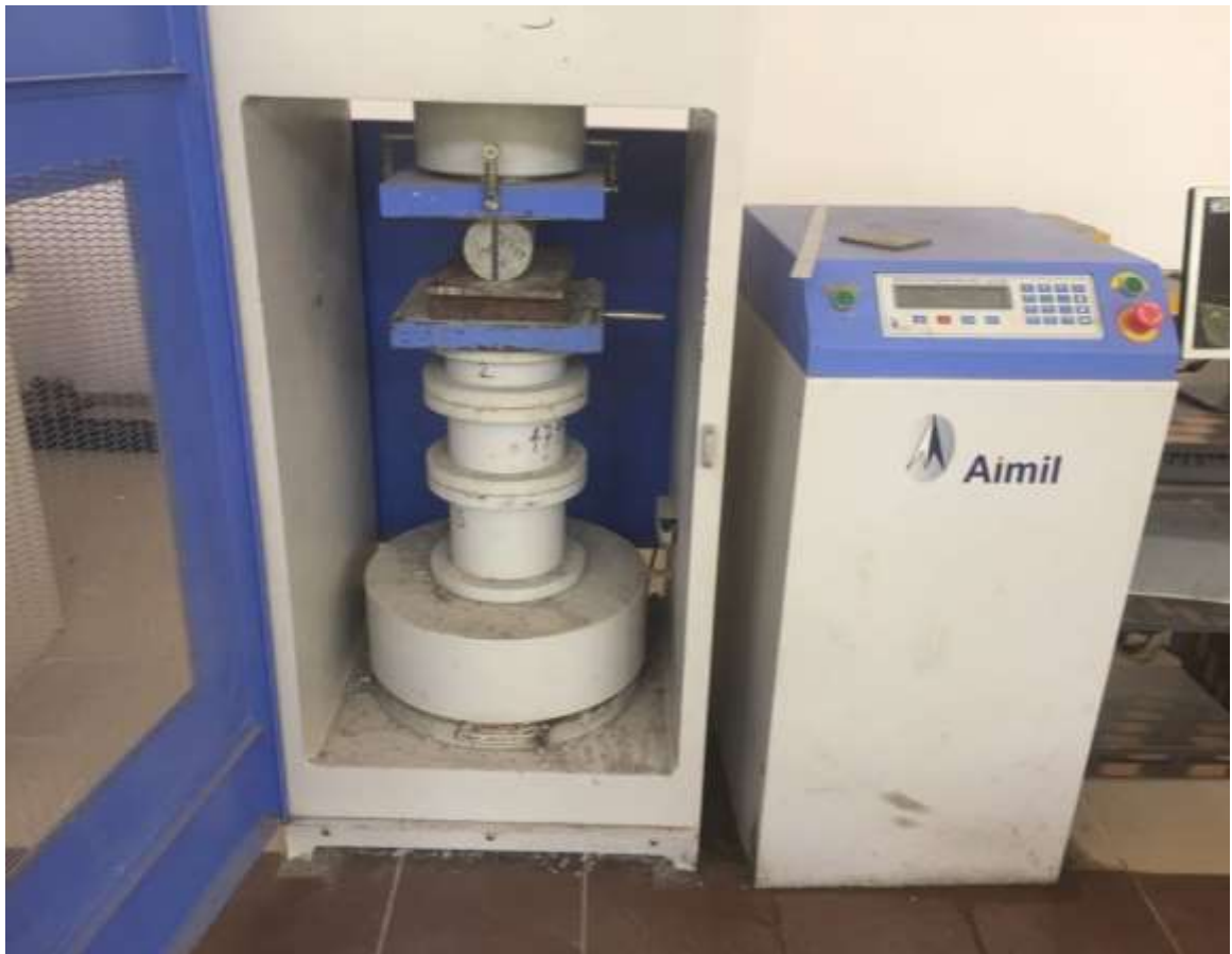
Fig 3.8: Splitting Tensile Strength using CTM
