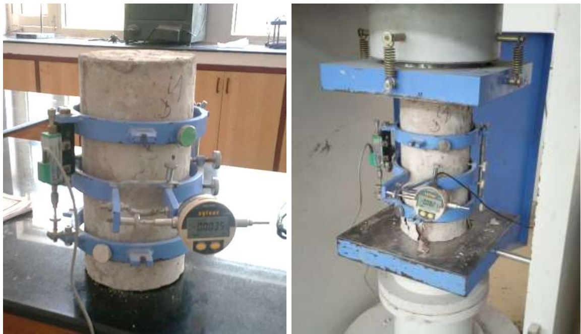
Fig 3.10: Frame Assembly for Modulus of Elasticity test.
