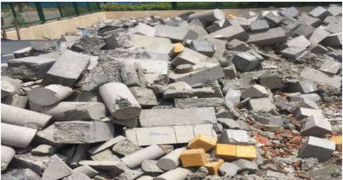
Fig 3.1: Laboratory waste used for producing FRCA
