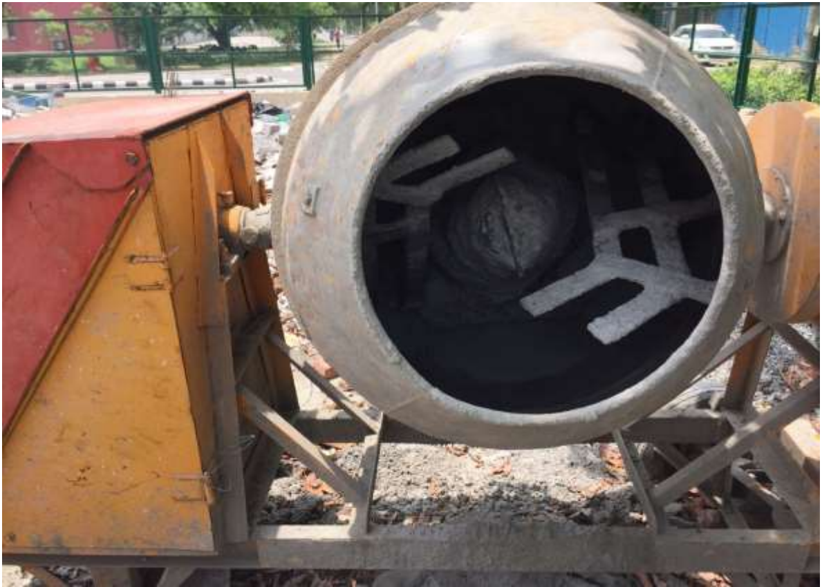
Fig 3.5: Concrete Mixing Machine.
