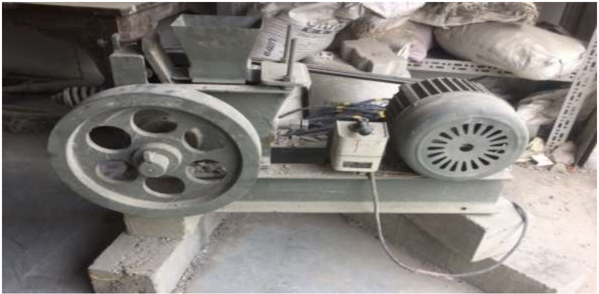
Fig 3.2: Jaw Crusher used to crush concrete waste from the laboratory.
