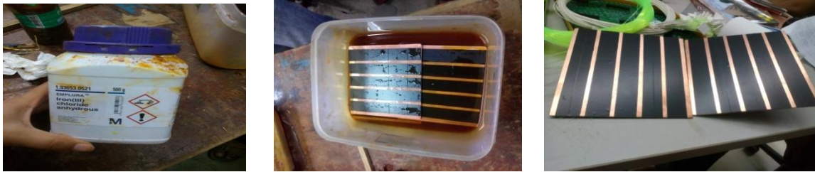
Figure 4.6: Steps showing fabrication of pick-up panels
