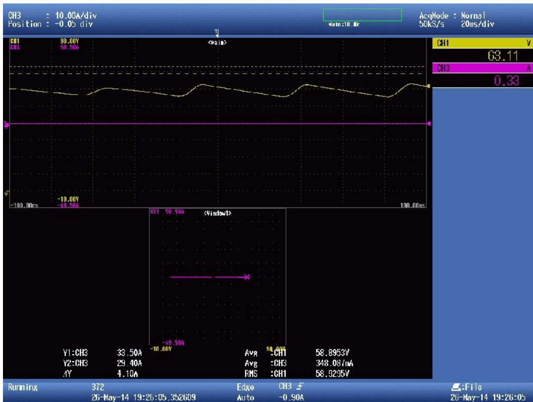
Figure22 Scope output for Open Circuit Condition.
