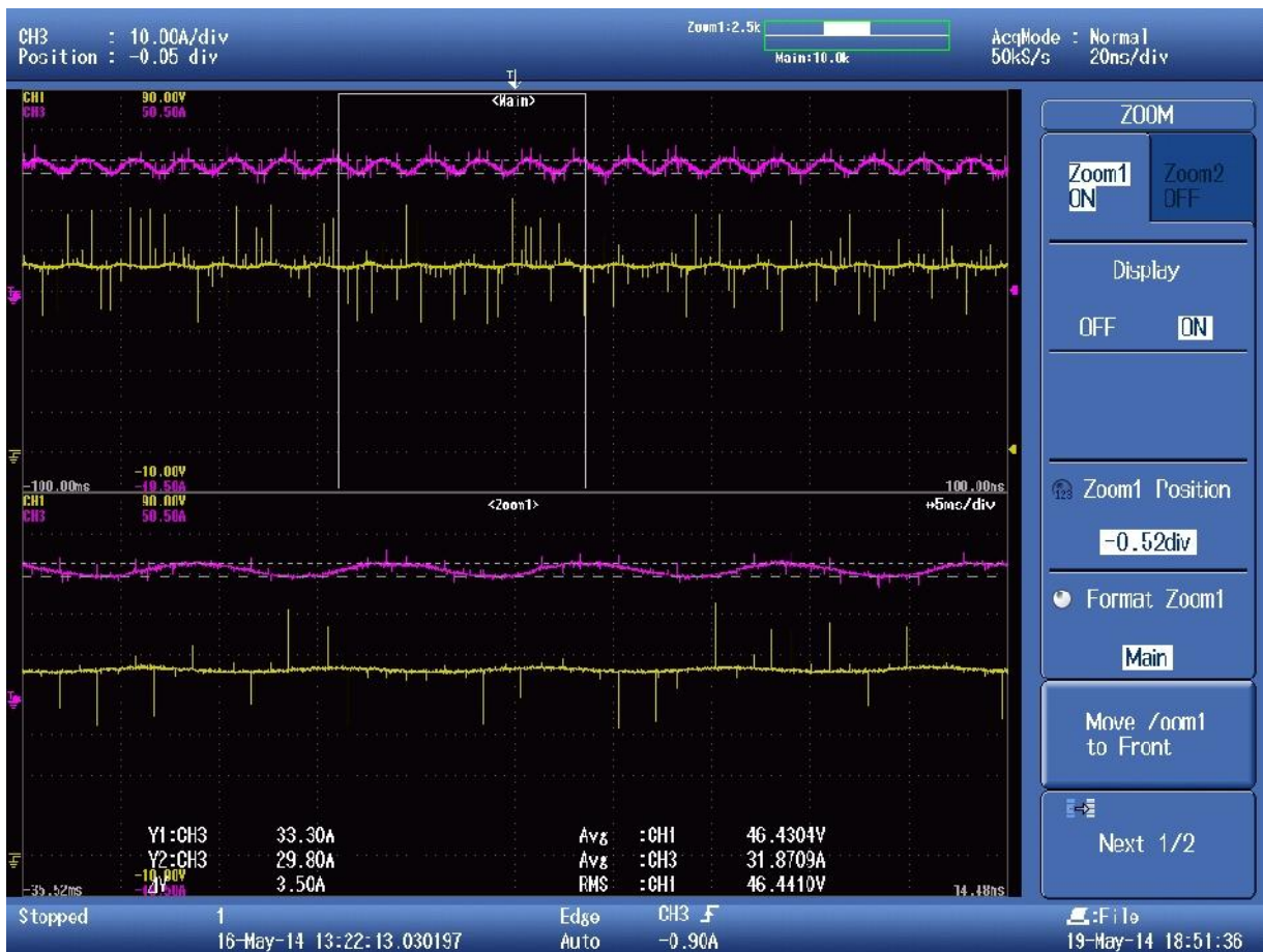
Figure25 Scope output of SAE at a load demand lower than MPP, i.e. 1.4kW.
