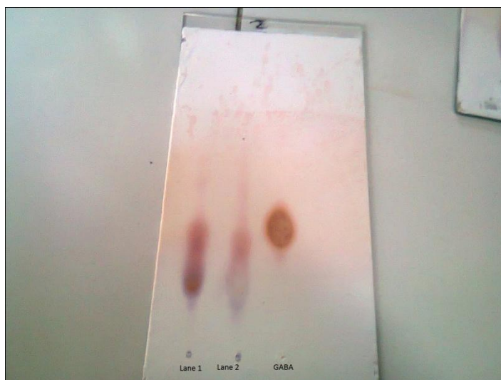
Fig 5.1-TLC chromatogram of standard and GABA production by L.lactis .
