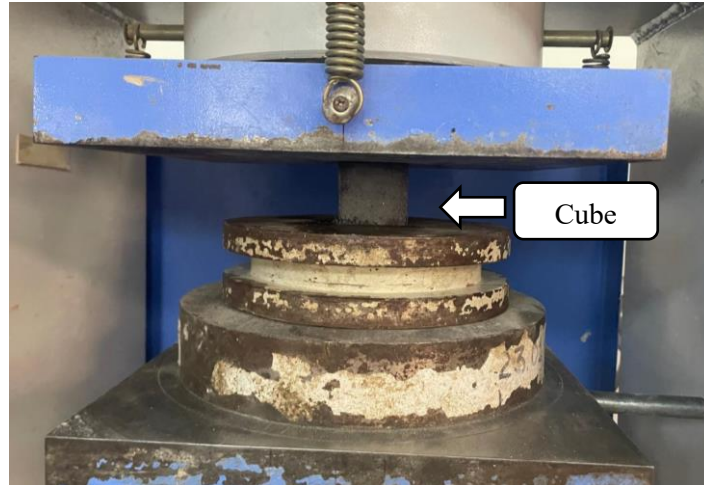
Fig3. 13 Compression testing of cube
