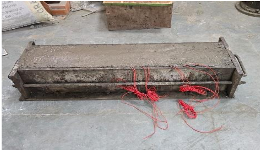
Fig3. 10 Beam after casting.
