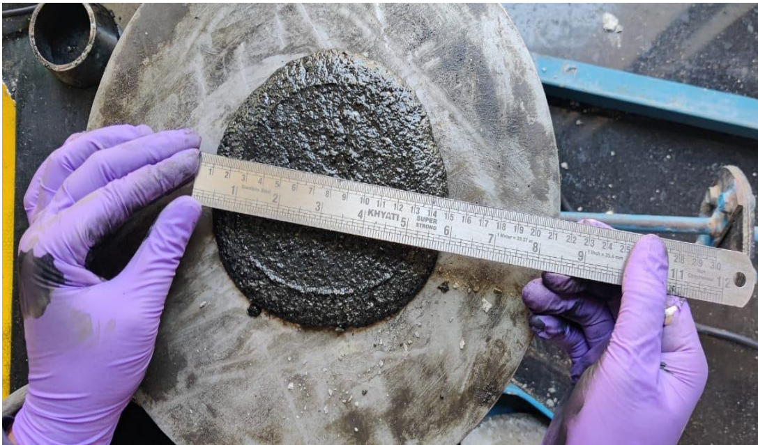
Fig3. 4 Measurement of flow using scale.
