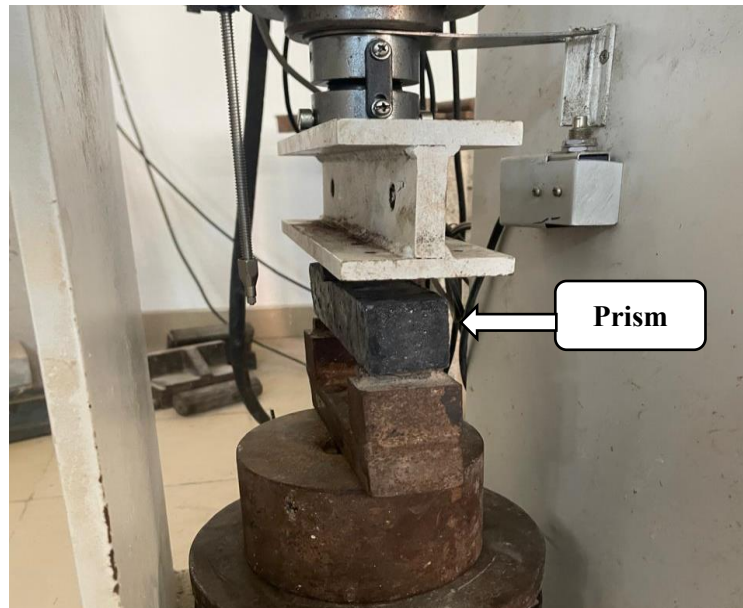
Fig3. 12 Flexural testing of prism
