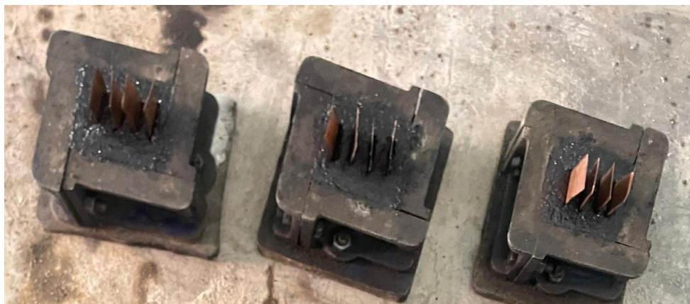
Fig3. 1 Copper plates embedment in cube samples
