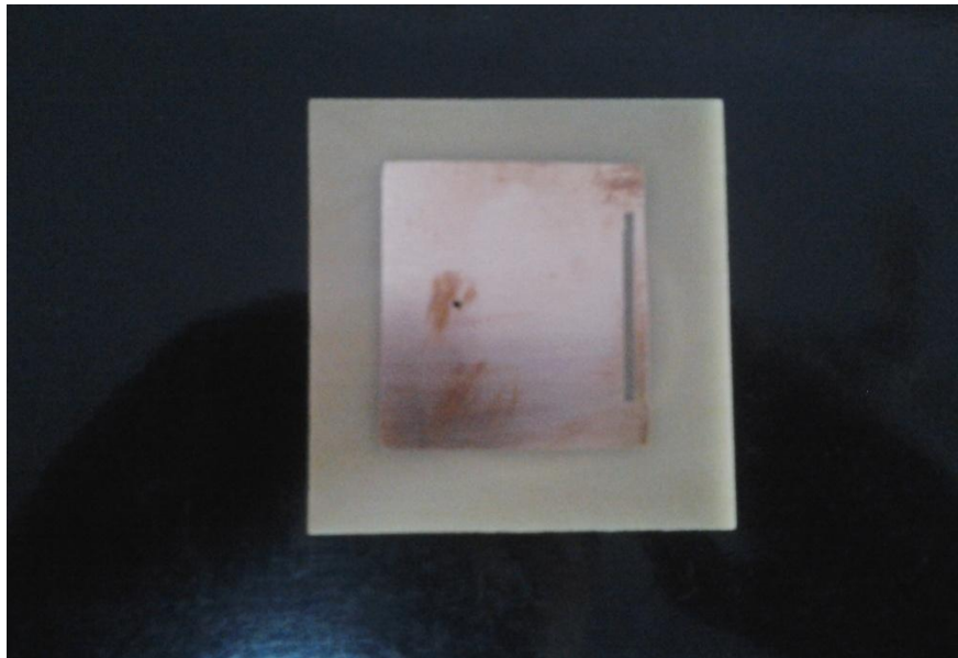
Fig 5.2: Fabricated antenna of coaxial fed dual band microstrip rectangular patch antenna for WLAN application
