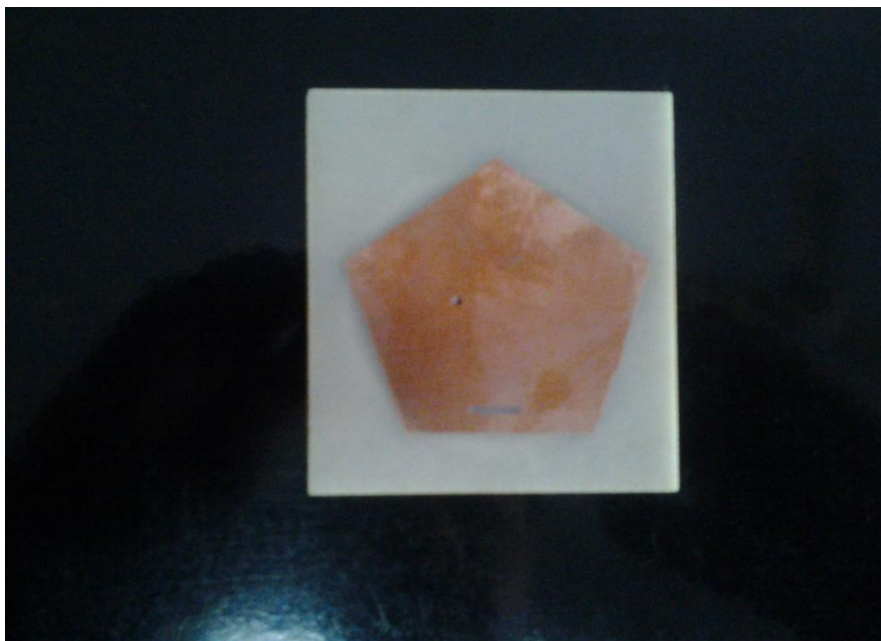
Fig 5.4: Fabricated antenna of coaxial fed dual band microstrip pentagonal patch antenna for WLAN application
