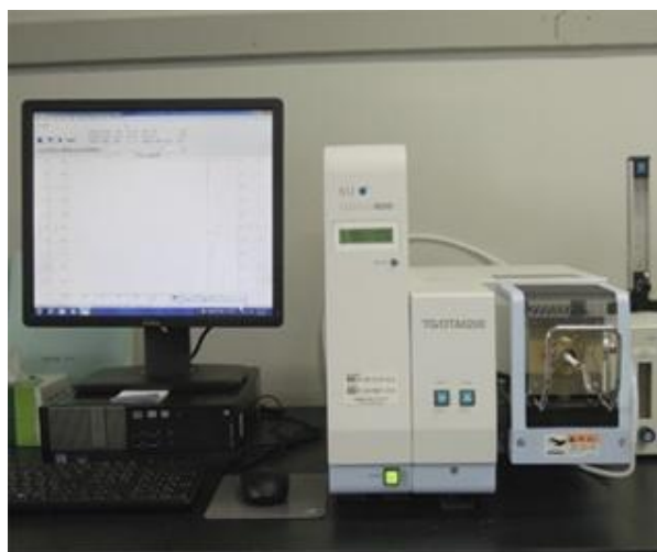
Figure 3.5: Differential Thermal Analyzer (DTA).
