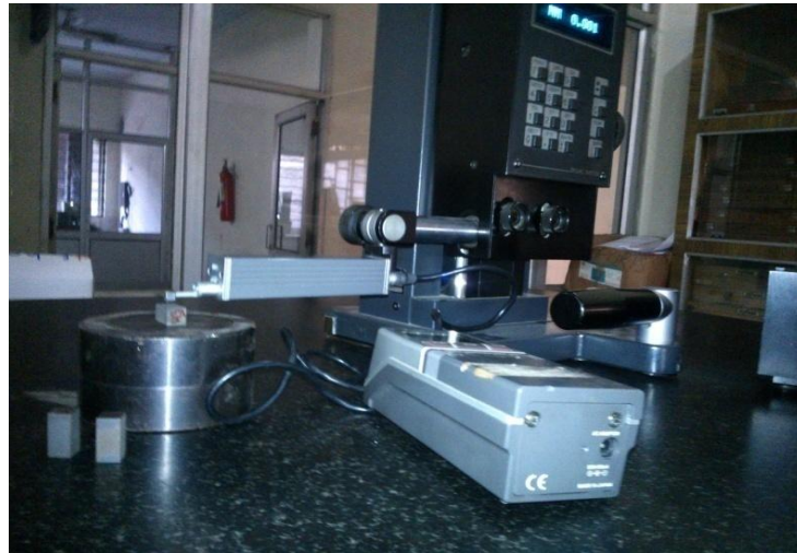
Figure 4.4 Set up for surface roughness measurement [ Model SJ-301, Source: Central Tool Room Ludhiana]
