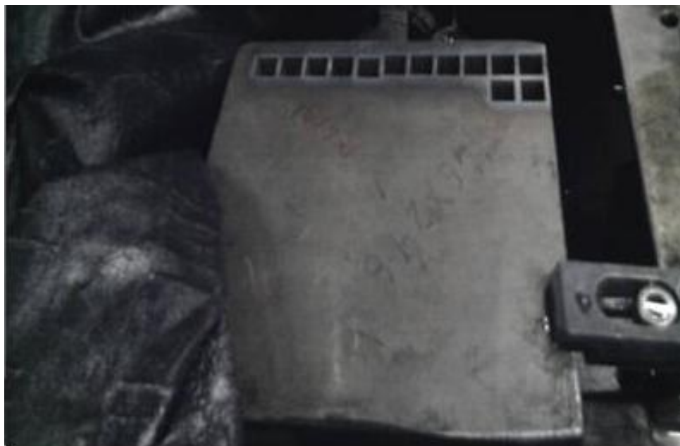
Figure 4.17 Complete job profile after WEDM
