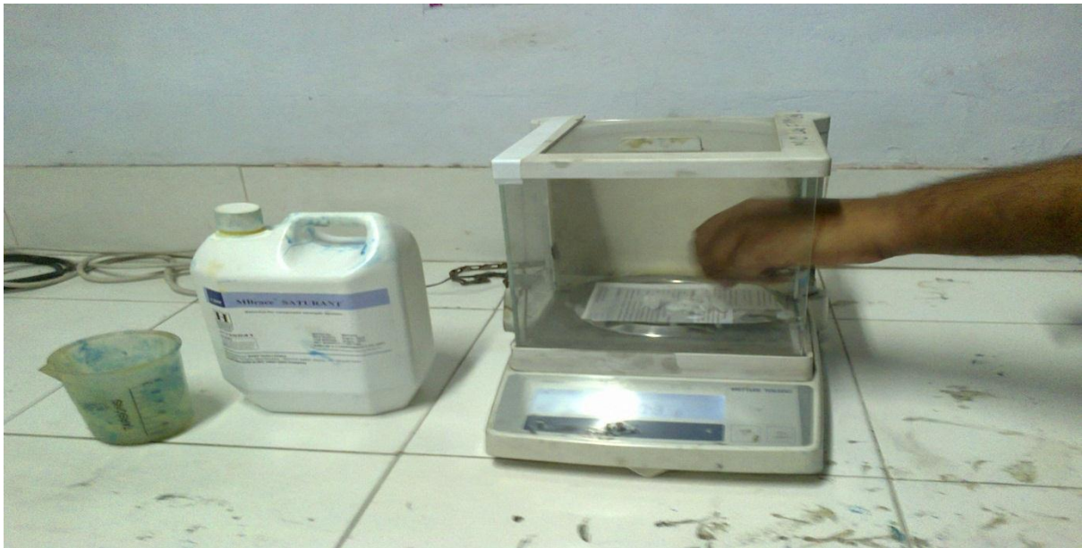
Fig 4.5 Weighing of Nano-clay, epoxy and hardner using digital weigh 'METTLER TOLEDO'
