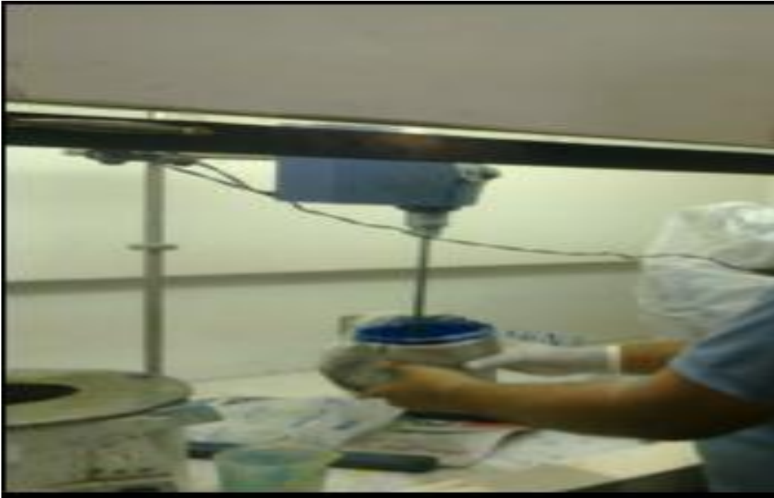
Fig 4.7 Homogeneously Mixing of Epoxy and Hardner
