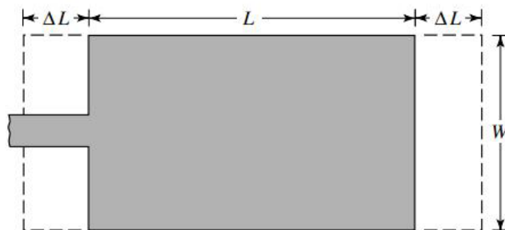
Fig. 1.6 Physical and effective length of MSA [3]
