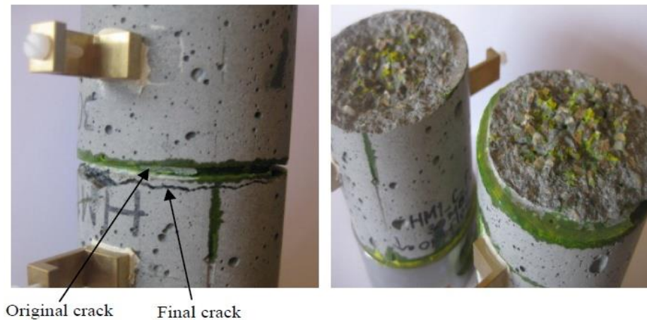
Figure 2.4: Original and final crack pattern after healing and new crack surface due to healing effect ( Sangadji et al., 2012 ).
