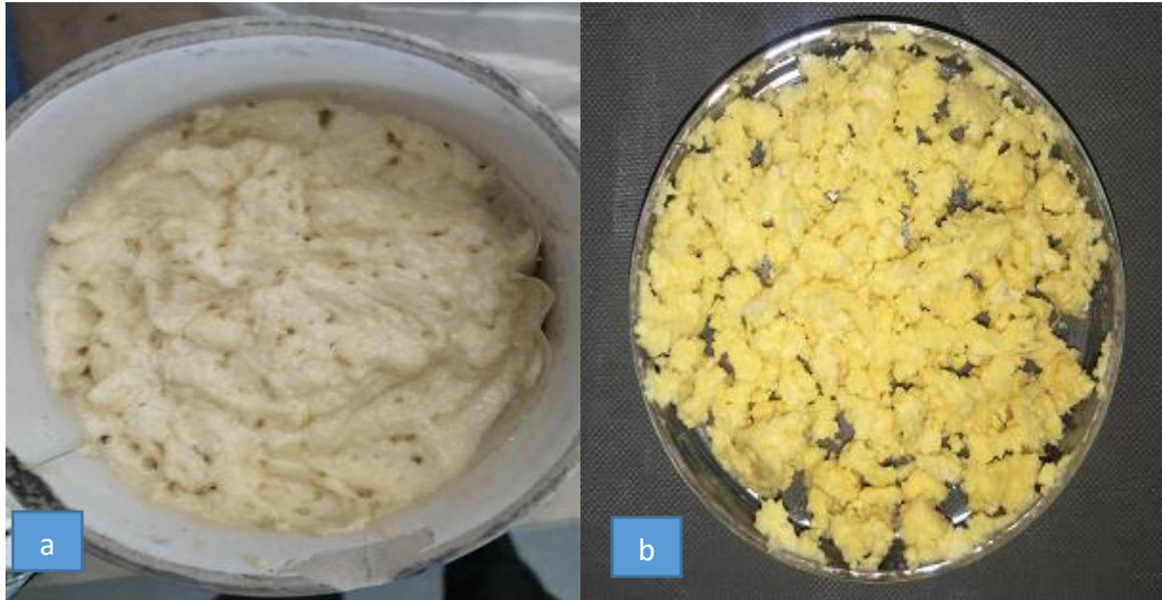
Figure 3.10: Tung-oil microcapsules; (a) Air dried microcapsules, (b) Oven dried microcapsules.
