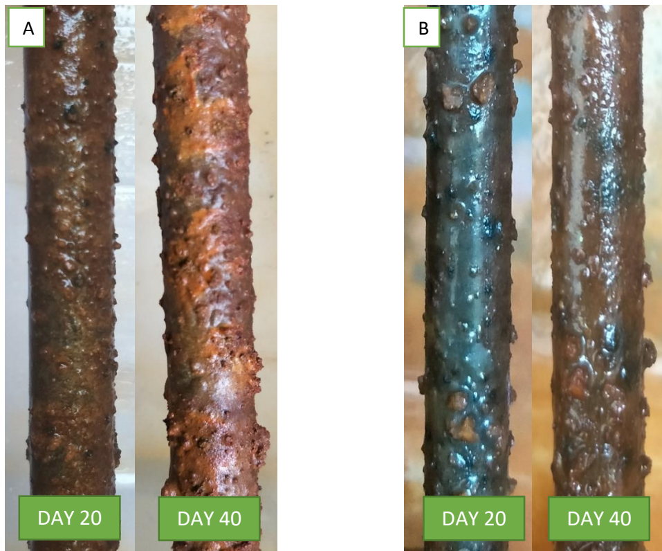
Figure 4.6: Visual observation, (A) MC-D rebar, (B) MNC-D rebar.
