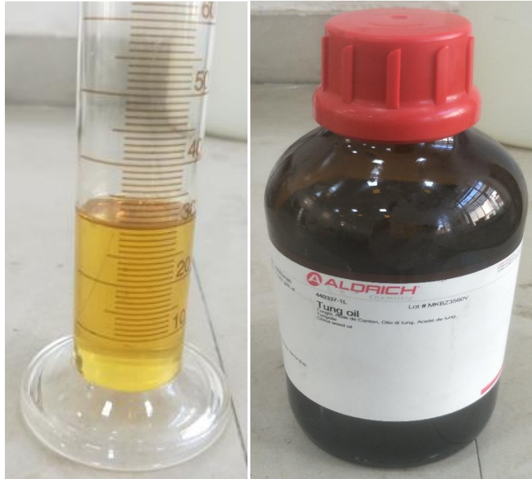
Figure 3.5: Self-healing agent, tung oil used in continuous phase.
