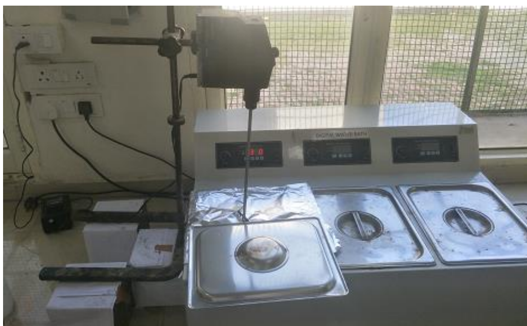
Figure 3.9: Covered solution for the polymerization reaction between Urea-Formaldehyde.
