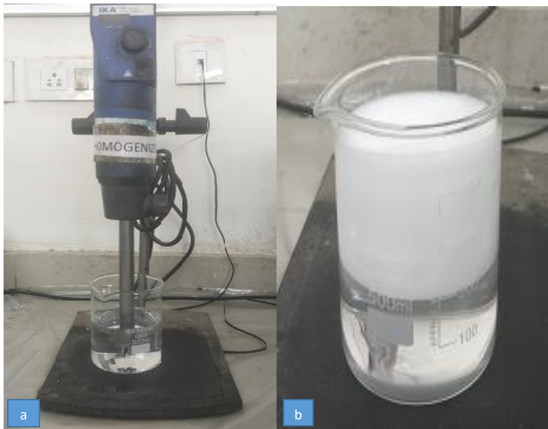
Figure 3.7: (a) Homogenizing of sample, (b) After homogenization.
