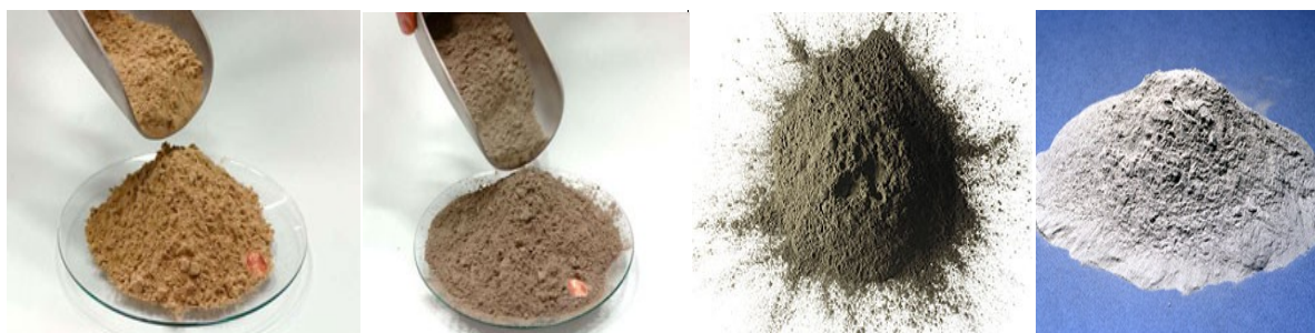
Figure 1.2.1b Variation in colour of fly ash depending on chemical and mineral constituents [40]
