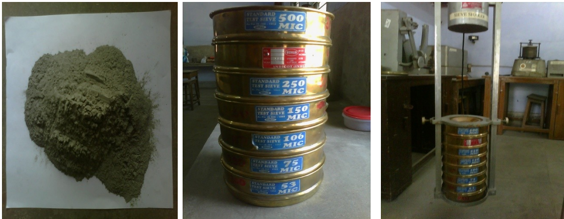
Figure 3.2.2 (a) Fly ash sample (b) Sieve system arrangement (c) Mechanical sieving machine.
