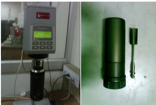
Figure 3.3.1 (a) Rheolab QC rheometer (b) Geometry used for measurements of higher concentration slurry.
