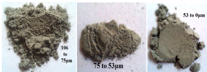
Figure 3.3.2f Visuals of particles less than 100 µm size
