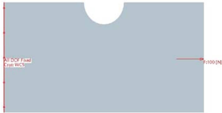
Figure 3.9(a) Beam fixed at one end and axially loaded at other end
