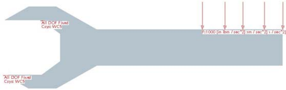
Figure 3.17(b) Boundary conditions and loading of the spanner
