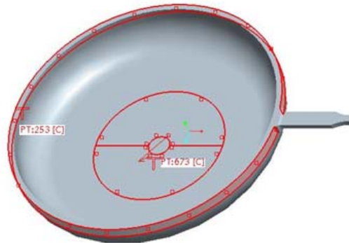
Figure 6.18(b) Boundary conditions and temperature fixation of the pan
