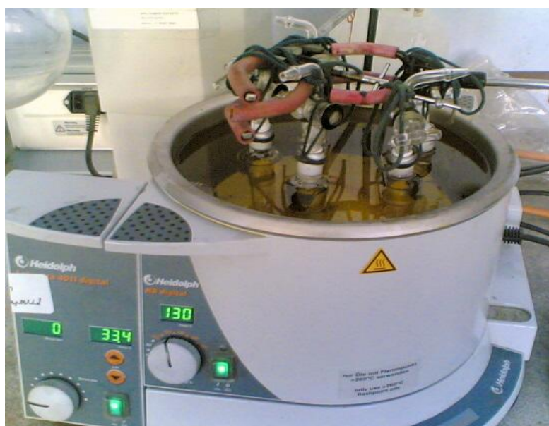
Figure 3.3 Experimental set-up for polymerization under vacuum
