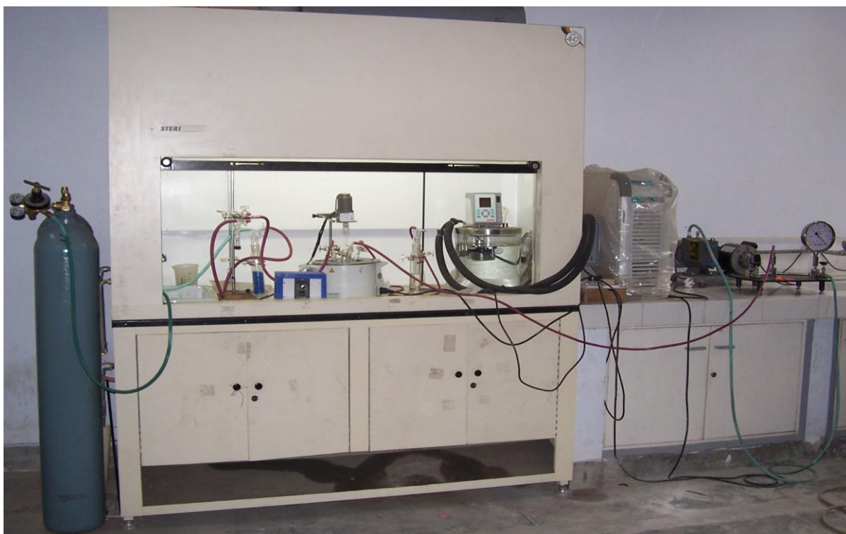
Figure 3.2 Experimental set-up for polymerization under nitrogen atmosphere
