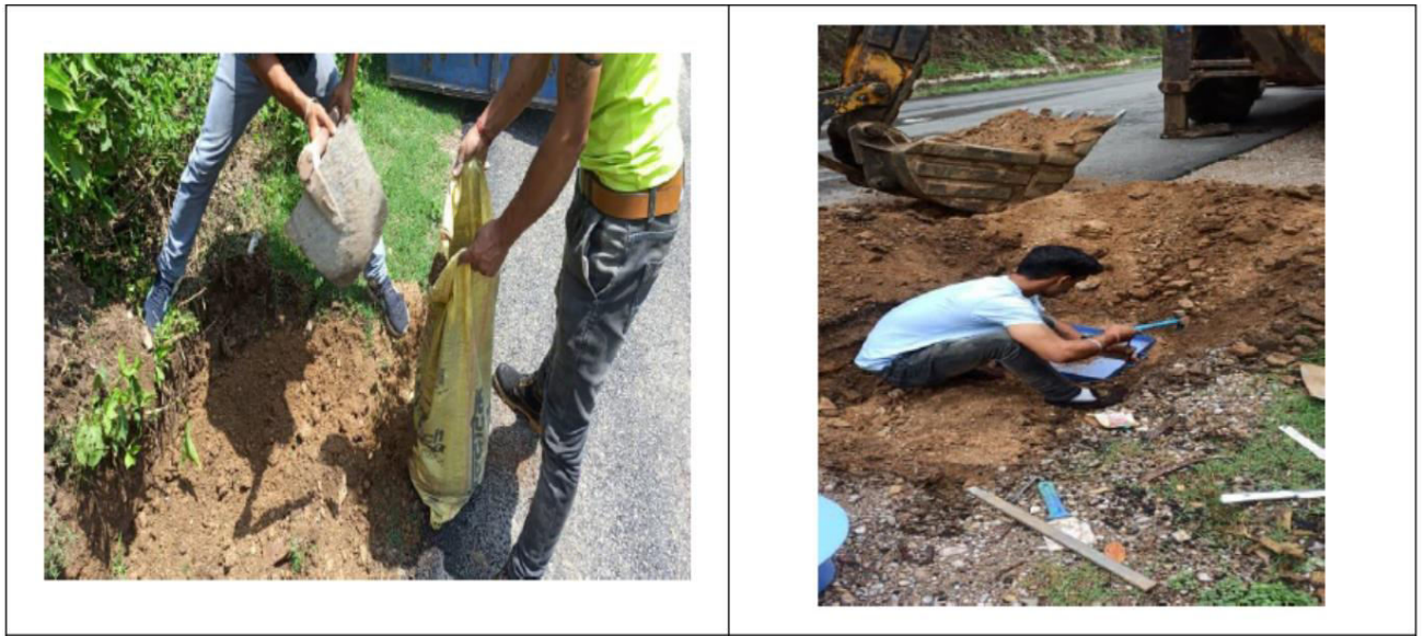
Fig. 3.16: Photos of test Pits Depicting Soil Sampling
