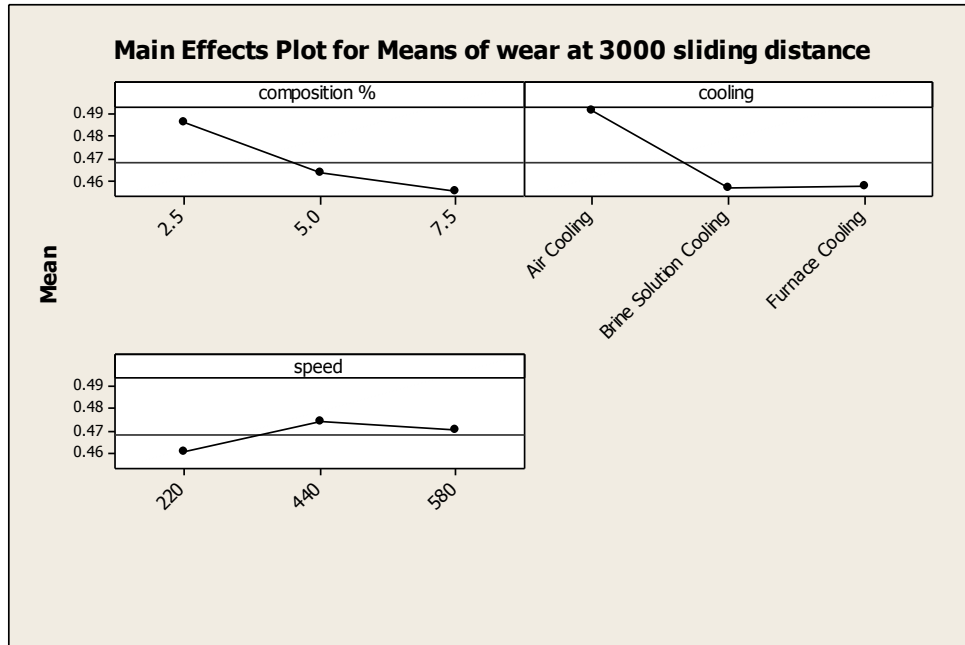
Figure 5.23: Main effect plot for Mean wear rate at 3000 sliding distance
