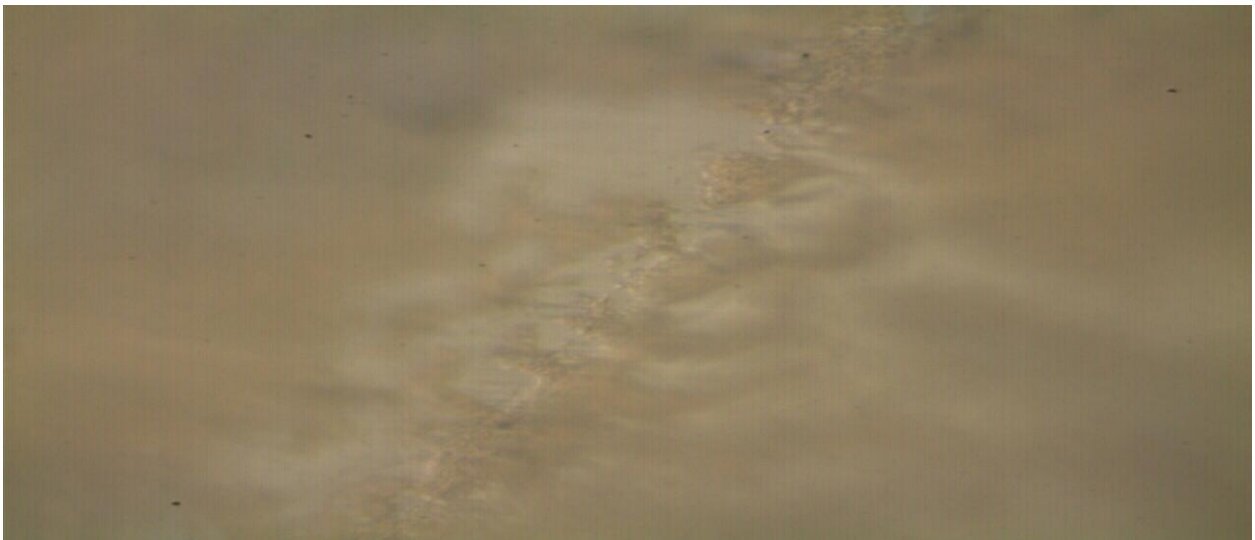
Figure 6.11: Optical micrograph of composite with 5% \text{Al}_2\text{O}_3 furnace cooled and 440 stirring speed at 50X
