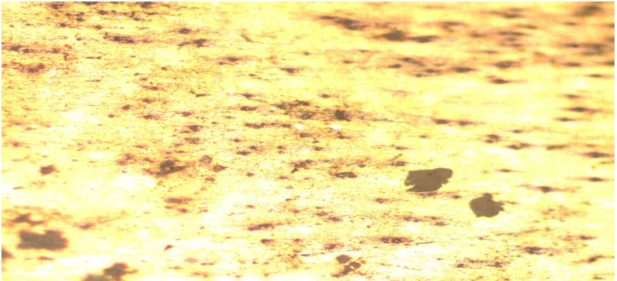
Figure 6.13: Optical micrograph of composite with 7.5% \text{Al}_2\text{O}_3 brine solution cooled and 440 stirring speed at 10X
