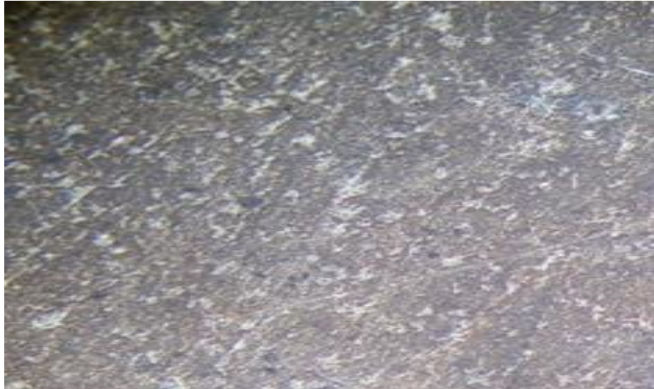
Figure 6.2: Optical micrograph of composite with 5% Al 2 O 3 air cooled and 440 stirring speed at 50X
