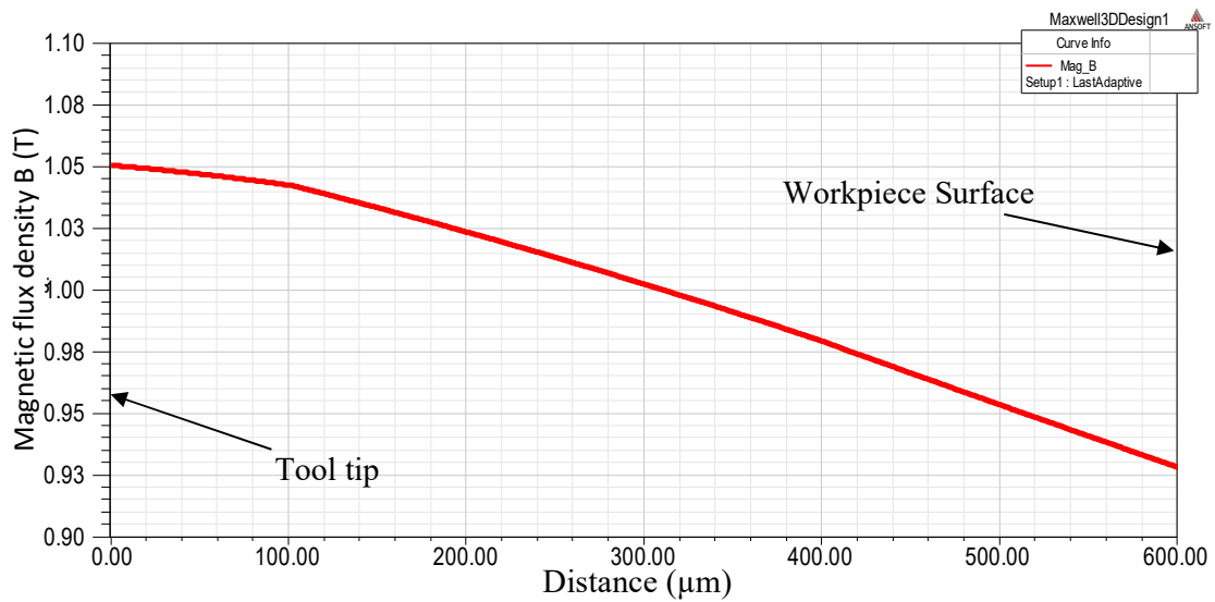
Figure 3.5 Magnetic flux density variation in the working gap along Z axis (Figure 3.4 (a))
