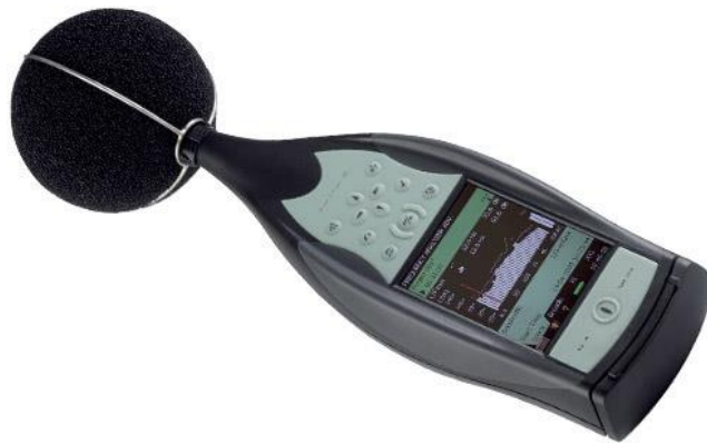
Fig. 1.1 An integrating type sound level meter with windscreen (B & K 2250)
