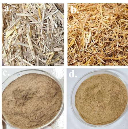
Figure 13: a. Non grinded WS, b. Non grinded RS, c. Grinded & sieved wheat straw (0.5 mm) d. Grinded & sieved rice straw (0.5 mm)
