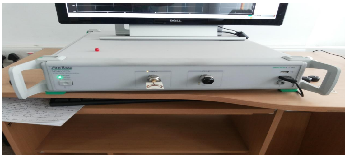
Fig. 5.4. Photograph of VNA and antenna connection.
