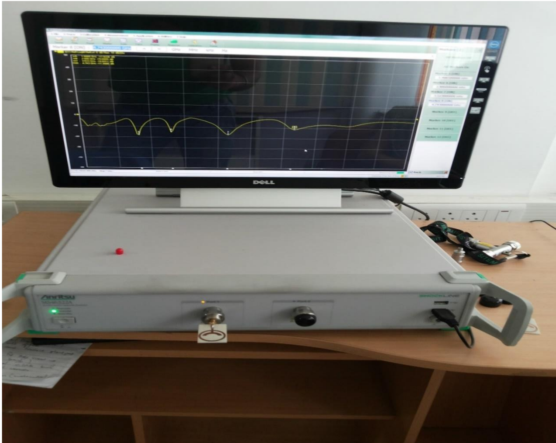
Fig. 5.5. Photograph of measured return loss of proposed antenna.
