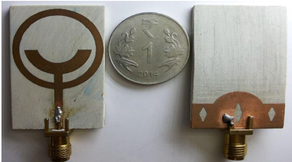
Fig. 5.3. The photograph of top and back view of the fabricated antenna.
