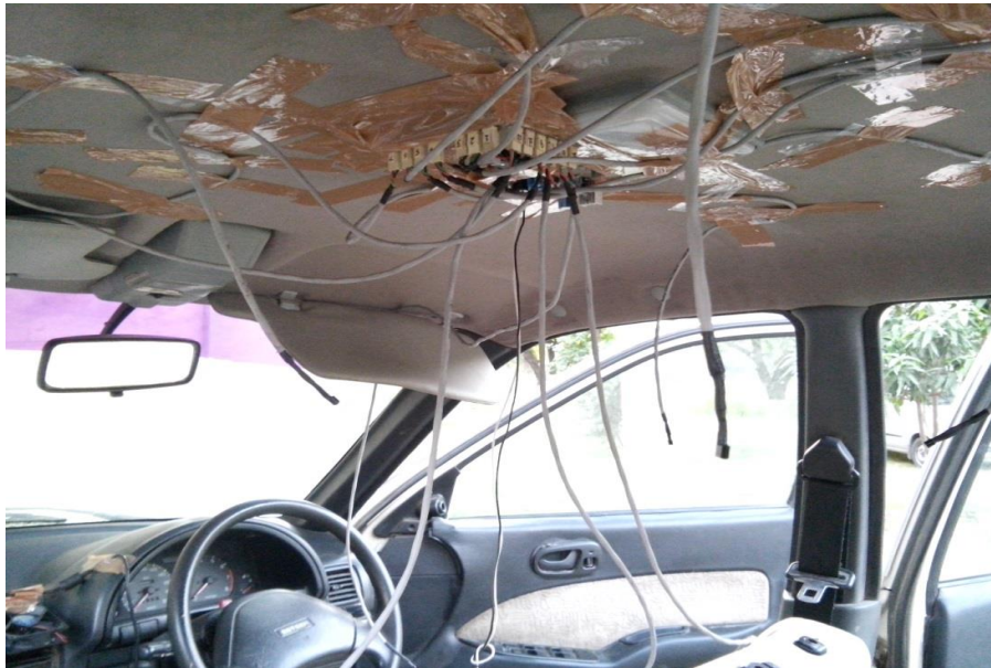
Figure 3.6 Placement of the PCB and sensors
