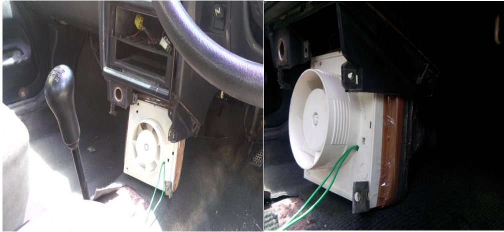
Figure 3.3 Fan installed in the front part of the car cabin
