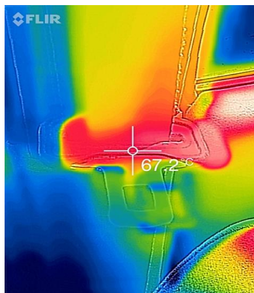
Figure 4.9 Thermal image of the seat belt
