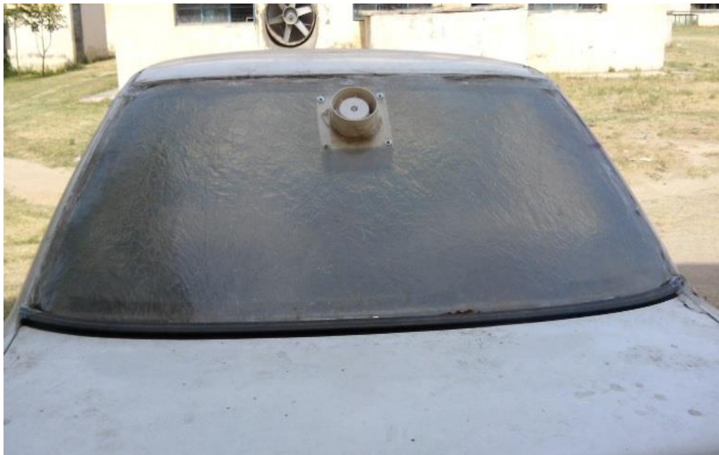
Figure 3.4 Fan installed on the rear windshield
