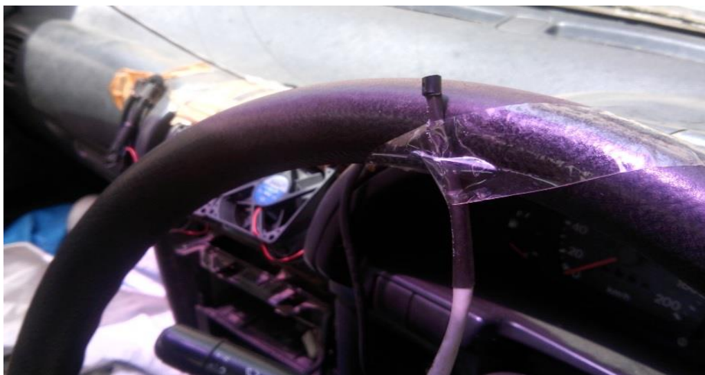
Figure 3.7 Placement of a sensor on the steering wheel
