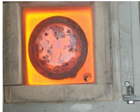
Figure 4.1.- Preparation of Samples in Electrical Resistance furnace
