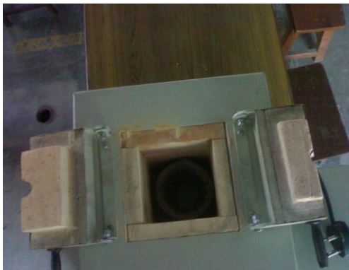
Figure 4.1.- Preparation of Samples in Electrical Resistance furnace
