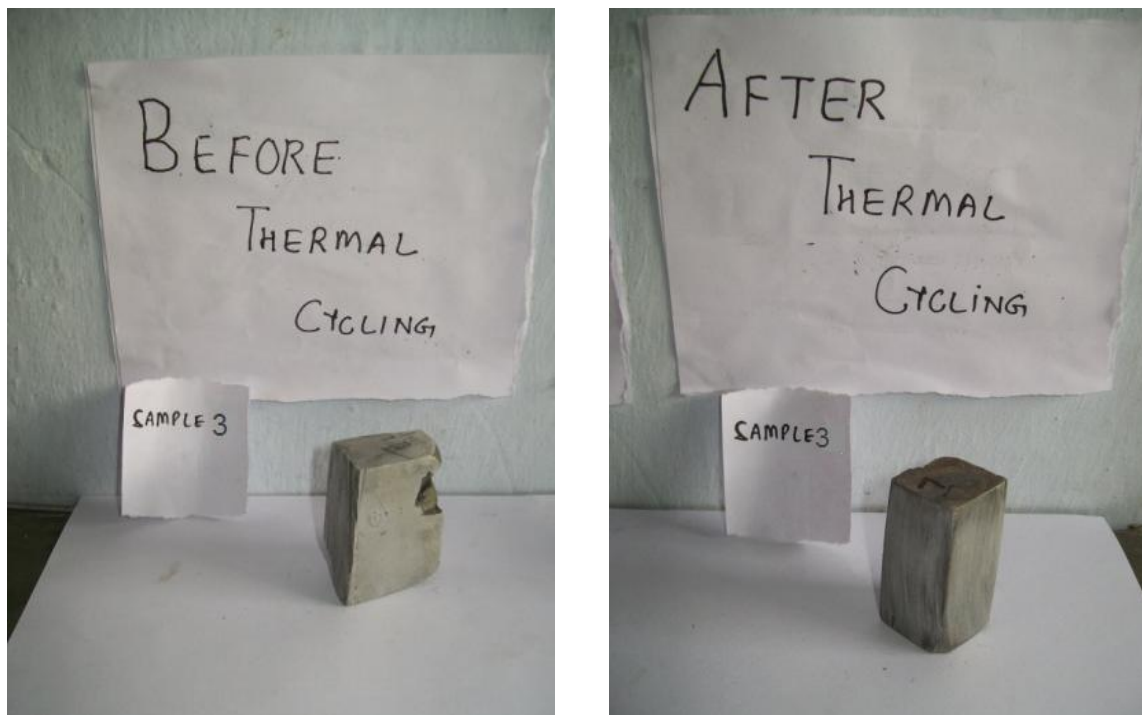
Fig 5.3- Pictures of Sample no.3 before and after Thermal cycling
