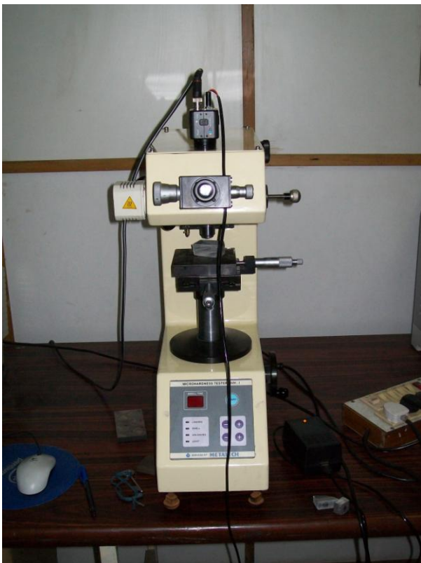
Figure 5.36- Pictorial view of Vicker's Microhardness Tester
