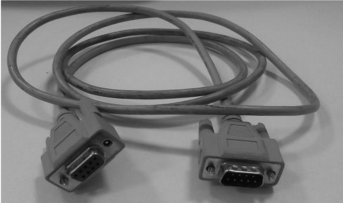
Figure 6.4: Serial cable used for connection of personal computer with Bluetooth module hardware.
