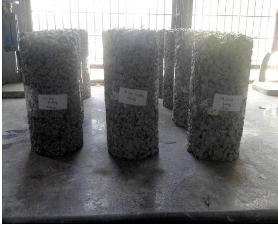
Fig. 3.9: Demoulded cylindrical samples
