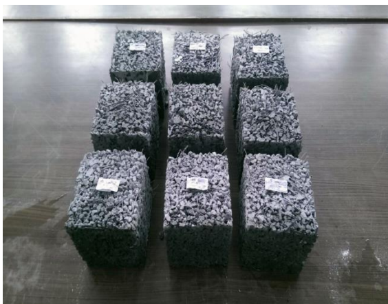
Figure 3.7: Demoulded cube samples
