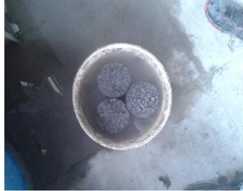
Fig. 3.18: Cylinders immersed in salt solution
