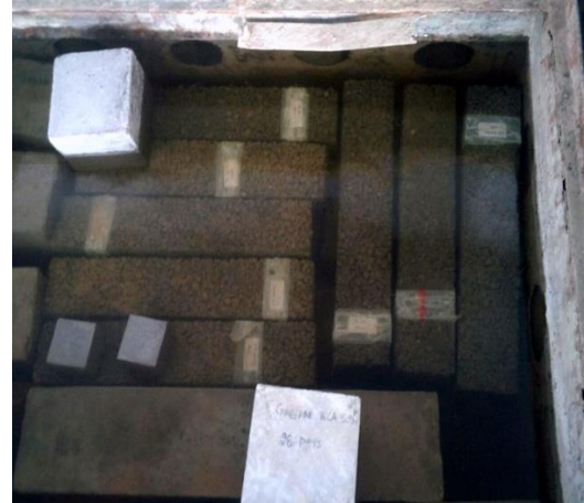
Fig. 3.10: Curing of beam samples in curing tank
