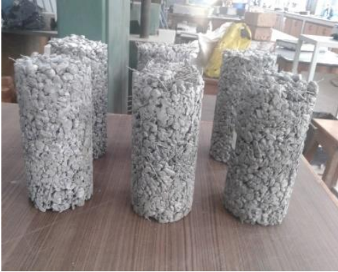
Fig. 3.17: Oven dried cylindrical specimen
