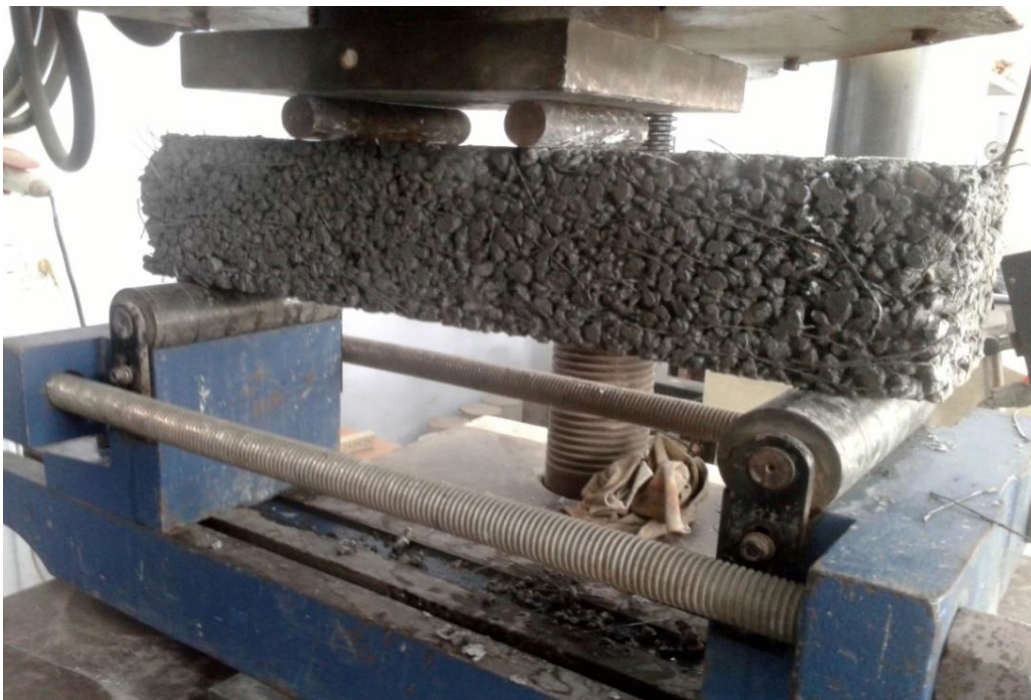
Figure 3.12: Two point loading test to evaluate flexural strength of Pervious Concrete beam
