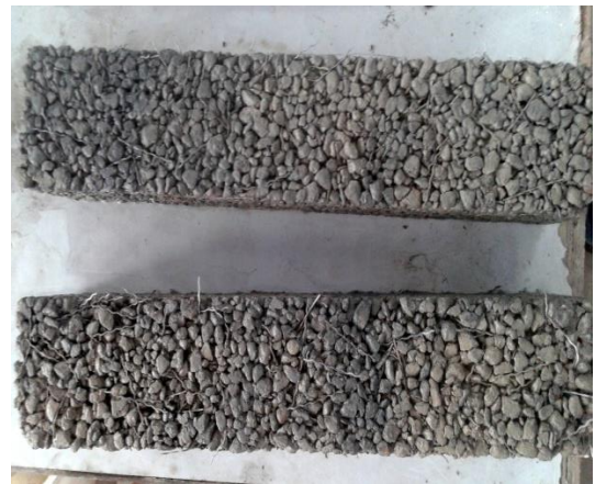
Figure 3.8: Demoulded beam samples
