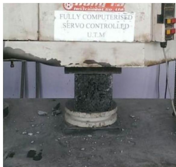
Figure 3.11: Compressive strength test on Pervious Concrete cube
