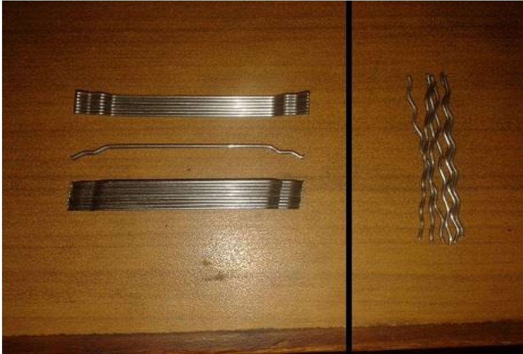
Figure 3.2: Different fiber types: Hooked end (4-D) fiber (left) and Round crimped fiber (right)
