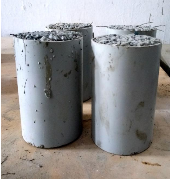
Figure 3.13: Pervious Concrete mould
