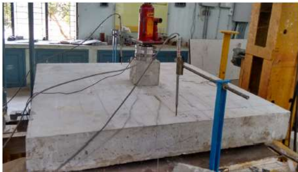
Figure 2.5: Concentrated load arrangement for the experiment (Daniel et.al (2018))
