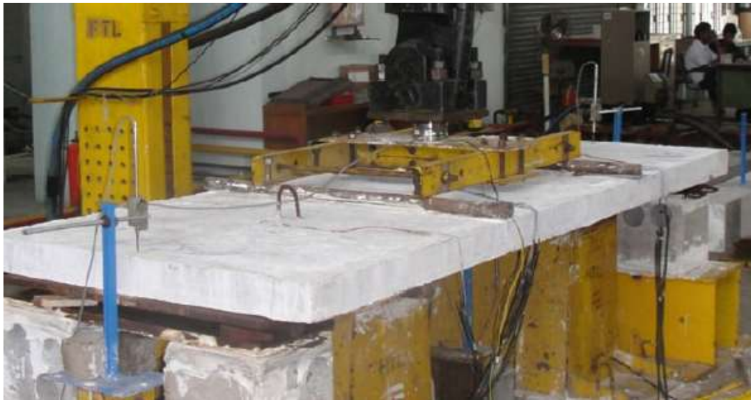
Figure 2.4: Four- point bend arrangement for the experiment (Daniel et.al (2018))
