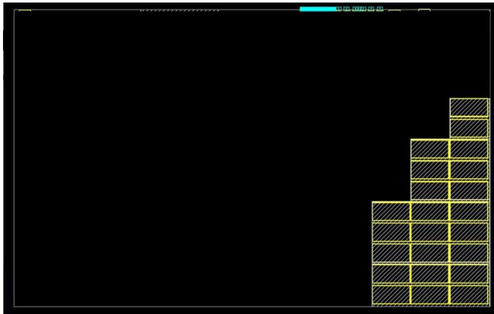
Fig. 7.1: Macro Placement in the assigned partition
