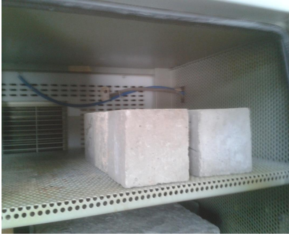
Fig 3.7: Cubes kept in Carbonation Chamber for Carbonation Depth Test
