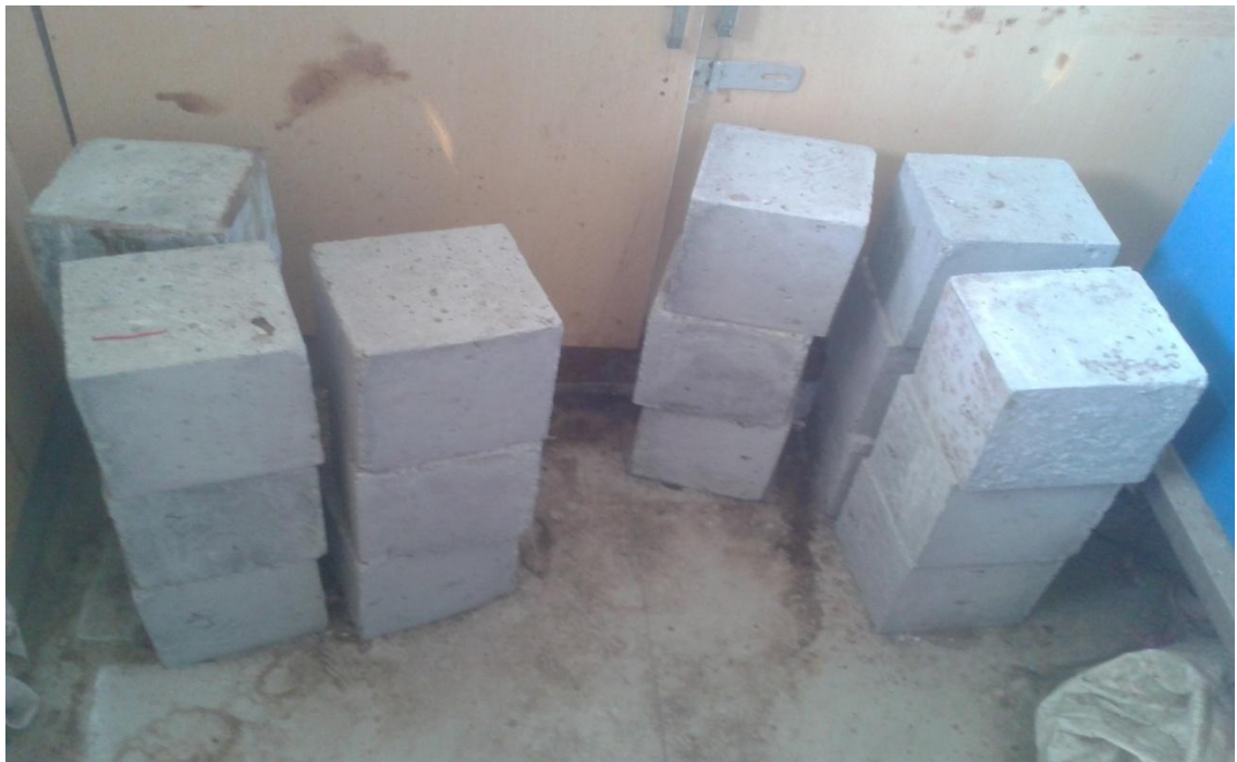
Figure 3.6: Cubes after casting for Compressive Strength Test
