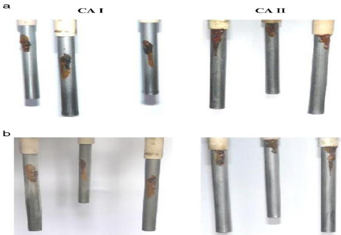
Figure 2.4: Images of steel samples: (a) after the corrosion initiation and (b) after the last addition of inhibitor for CA I and CA II tests (Królikowska et al, 2011)
