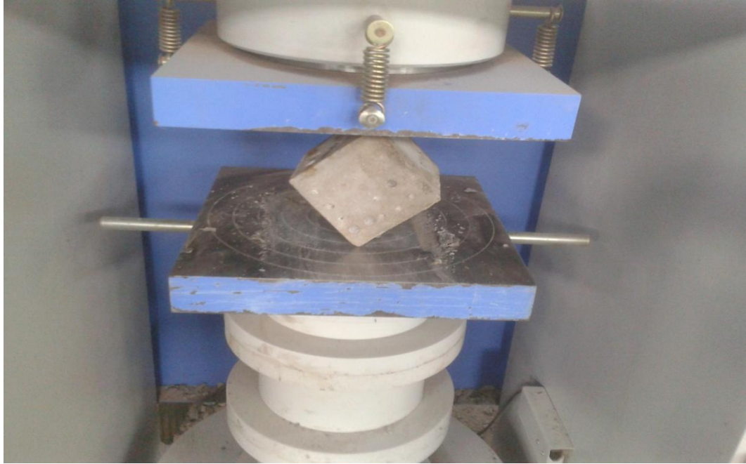
Figure 3.11: Set Up for Carbonation Depth Test
