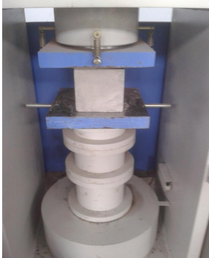
Figure 3.9: Set Up for Compressive Strength Test
