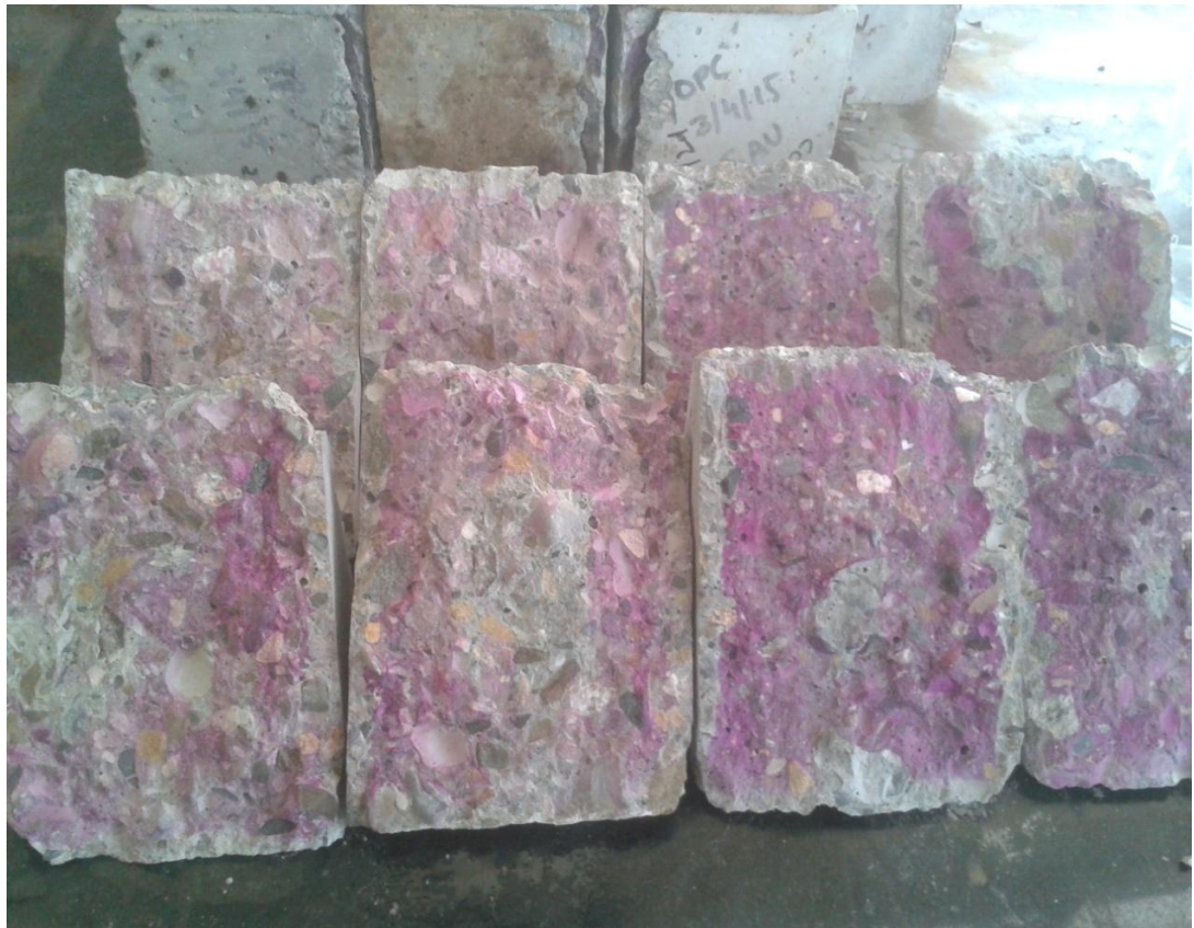
Figure 3.12: Cubes after the application of Phenolphthalein Solution
