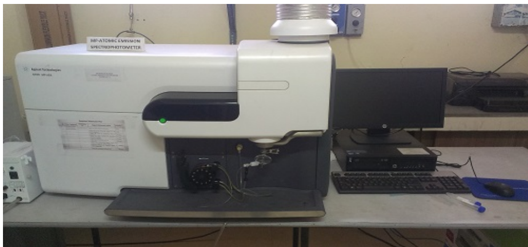
Figure 4.25: MP-AES apparatus [SAI Laboratories, Thapar University, Patiala]
