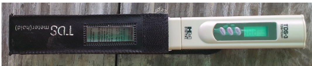
Figure 4.23: HM Digital made TDS meter [Energy laboratory, Thapar University, Patiala]
