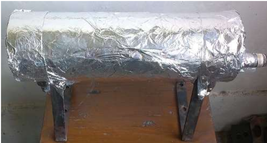
Figure 4.17: Water cooled condensing unit
