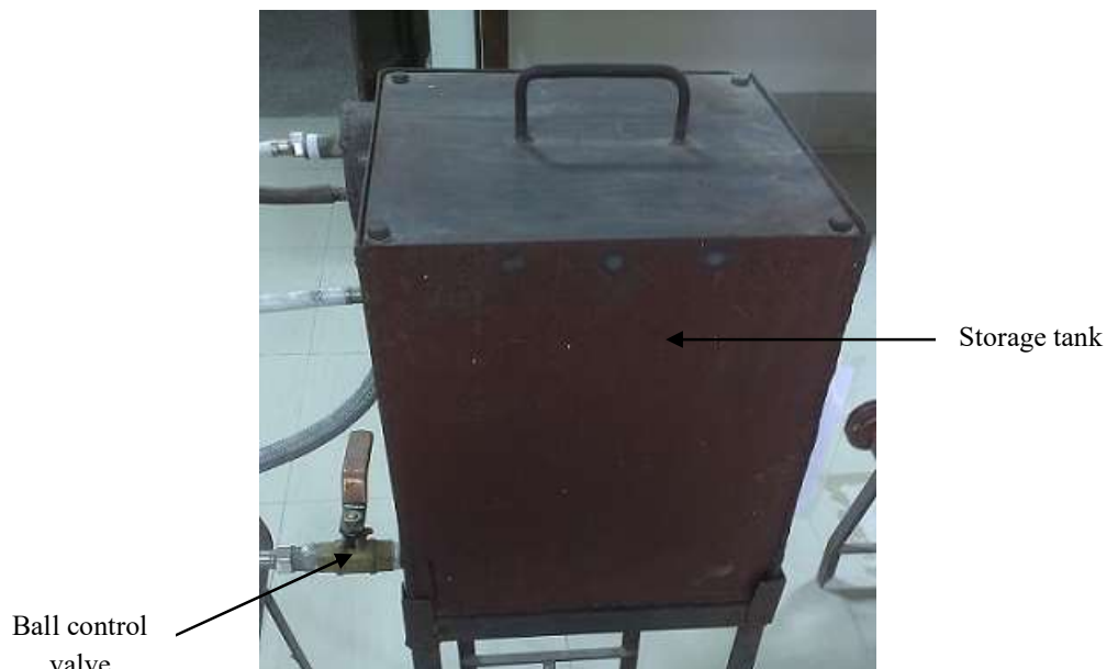
Figure 4.19: Hot ground water storage tank
