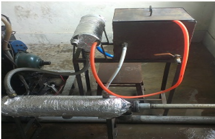
Figure 4.13: Photograph of the water purification unit
