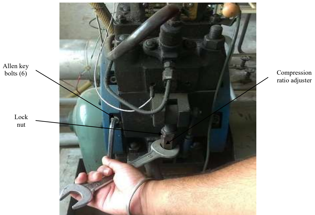
Figure 4.15: Mechanism to change compression ratio of VCRE
