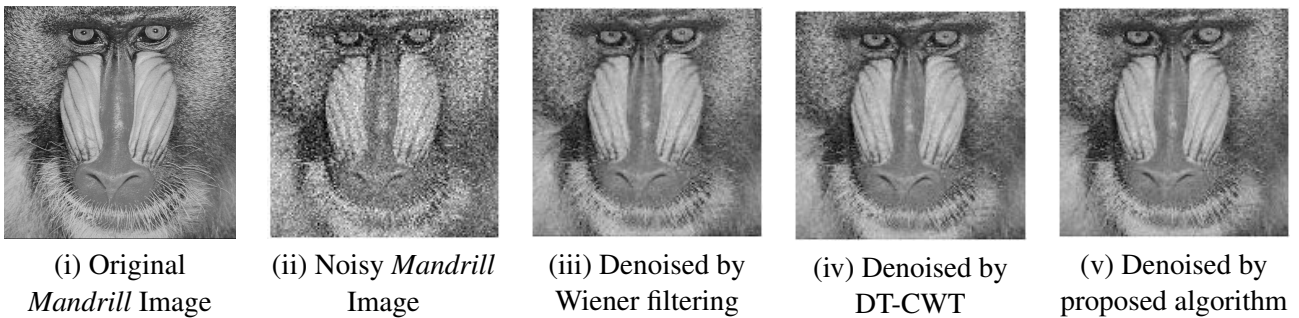
Figure 6.14: Noise standard deviation=35, PSNR=25.7063, PSNR=26.8050 and PSNR=28.0255
