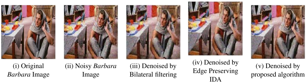
Figure 5.1: Noise standard deviation=15, PSNR=31.5256, PSNR=32.8907 and PSNR=34.7143
