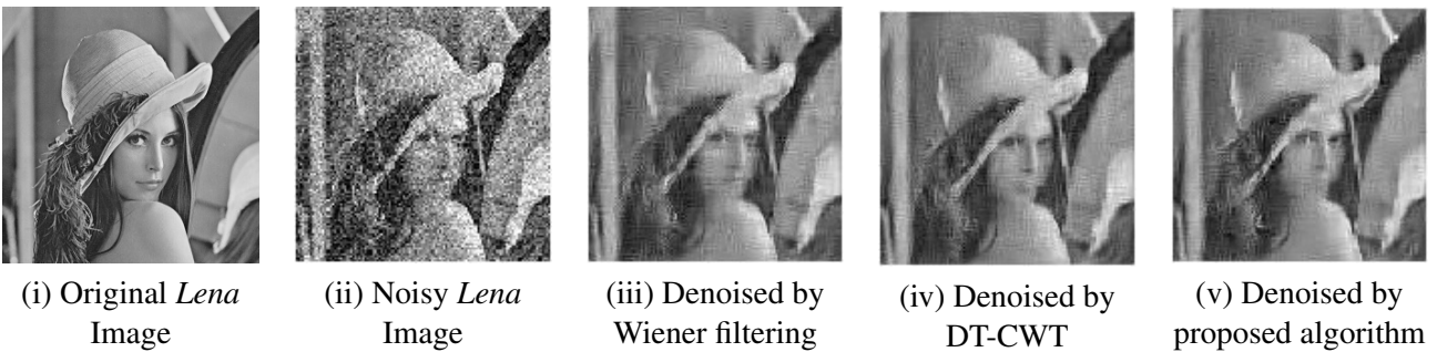
Figure 6.11: Noise standard deviation=35, PSNR=24.7809, PSNR=26.2505 and PSNR=28.0037
