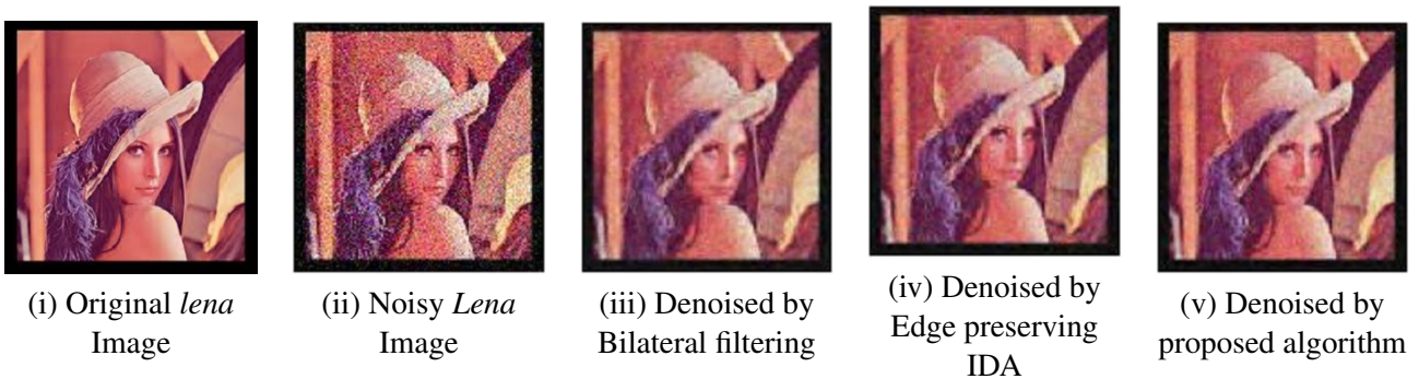
Figure 5.9: Noise standard deviation=35, PSNR=26.3869, PSNR=27.4536 and PSNR=28.9104
