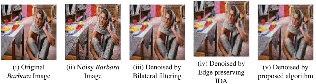
Figure 5.3: Noise standard deviation=35, PSNR=25.9062, PSNR=27.2269 and PSNR=28.5137
