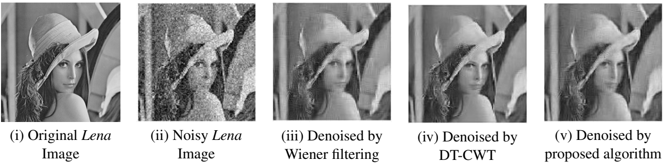
Figure 6.10: Noise standard deviation=25, PSNR=27.4792, PSNR=29.2165 and PSNR=31.0314
