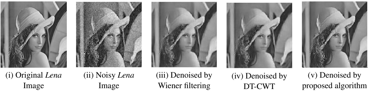
Figure 6.9: Noise standard deviation=15, PSNR=30.8312, PSNR=32.3733 and PSNR=34.2148
