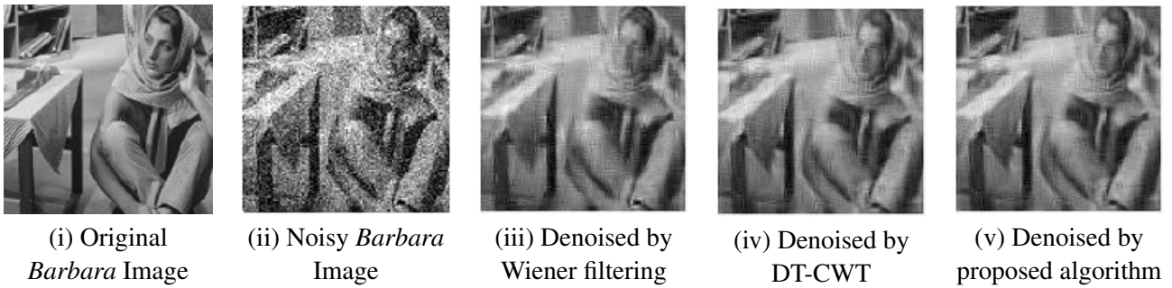
Figure 6.5: Noise standard deviation=35, PSNR=25.5809, PSNR=27.2405 and PSNR=28.6460
