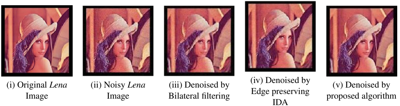
Figure 5.7: Noise standard deviation=15, PSNR=32.4323, PSNR=33.6932 and PSNR=34.8781
