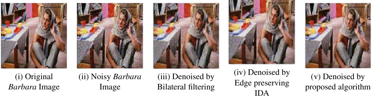
Figure 5.2: Noise standard deviation=25, PSNR=28.4294, PSNR=29.9428 and PSNR=31.1374
