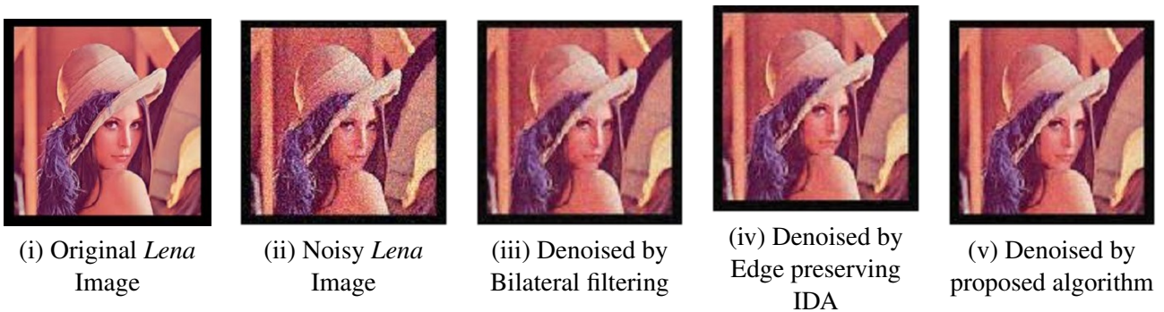
Figure 5.8: Noise standard deviation=25, PSNR=29.6861, PSNR=30.7365 and PSNR=31.9752
