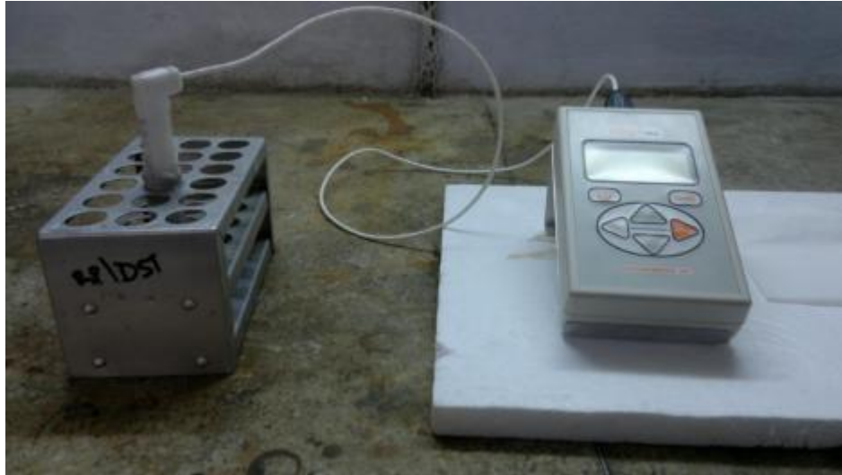
Fig 5.9 Measurement of thermal conductivity
