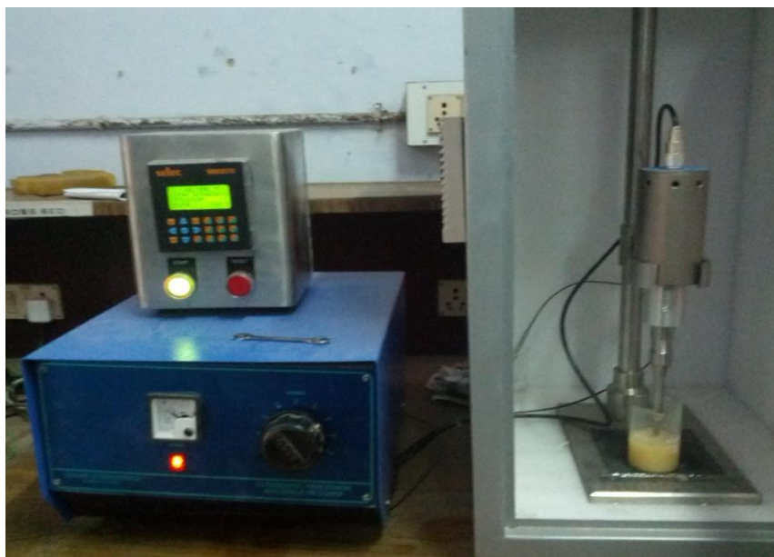
Figure 5.8 Sonication of sample in Ultra Sonicator
