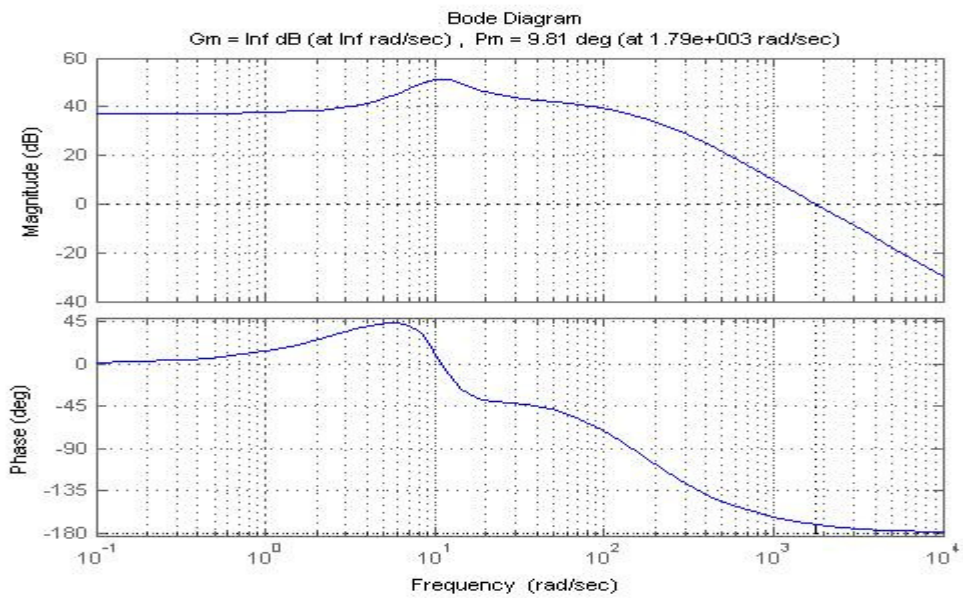
Figure 6.7(b): Bode Plot of Ideal PID controller with industrial controller
