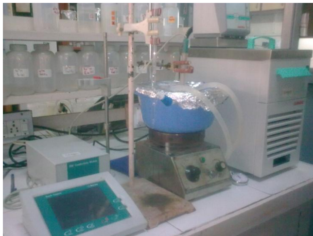
Figure 3.2: Experimental setup used for conductometric titrations
