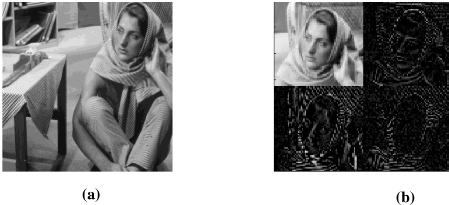
Figure 2.7: Implementation of DWT on Barbara Image (a) Barbara Image; (b) First level DWT decomposition of Barbara image
