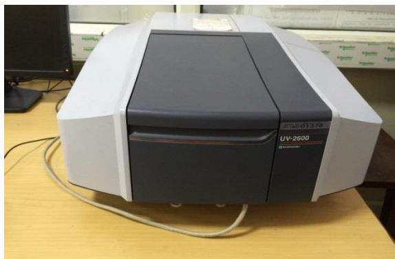
Figure 2.8 Pictorial view of UV-visible spectrophotometer.
