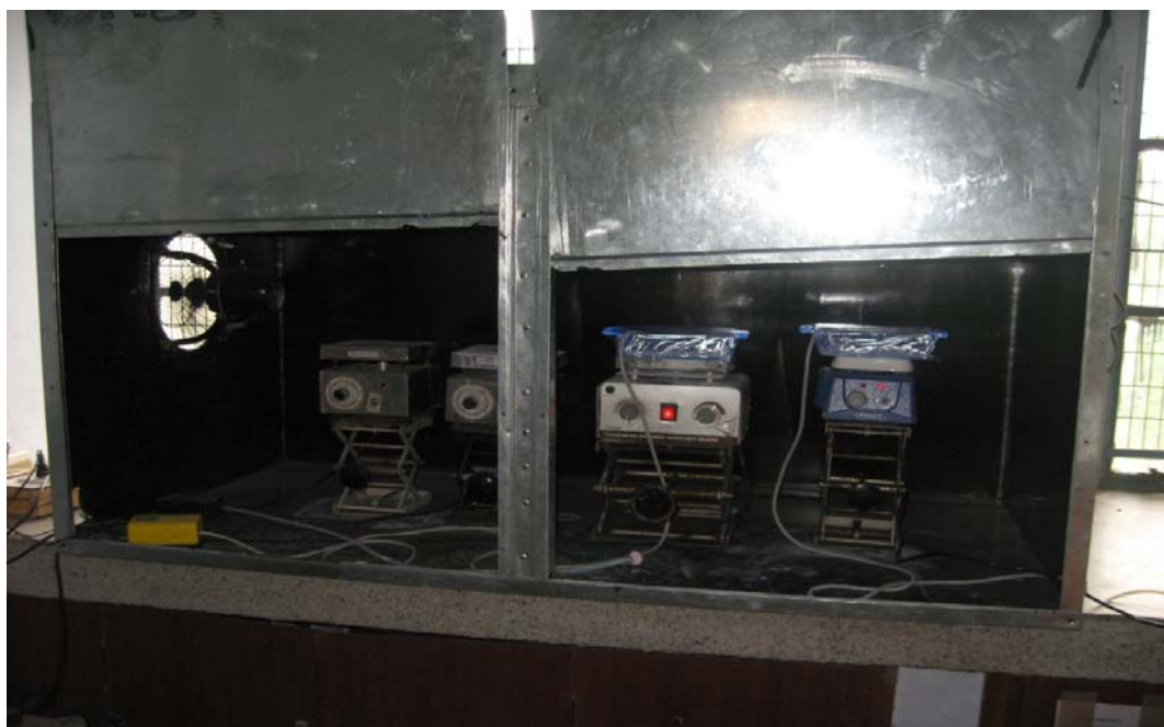
Fig-5.2 Photo reactor at lab level during photocatalytic treatment
