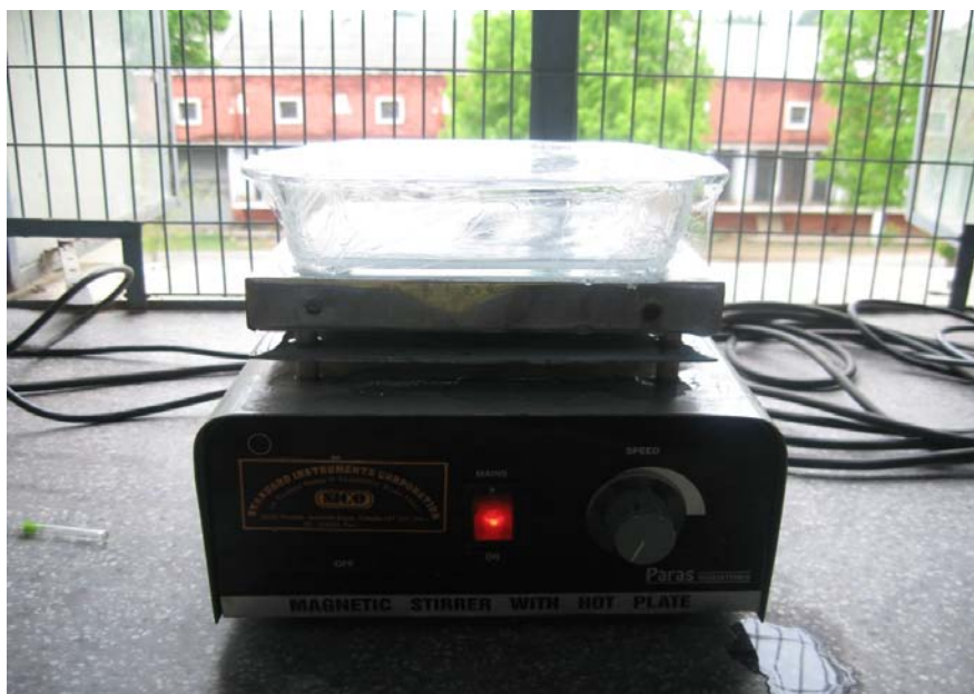
Fig: 5.3 Reaction vessel with magnetic stirrer during Photocatalytic treatment.
