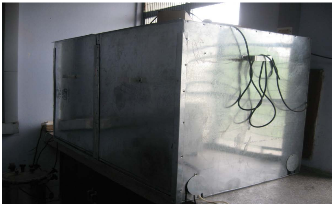
Fig- 5.1 Outer view of photo reactor
