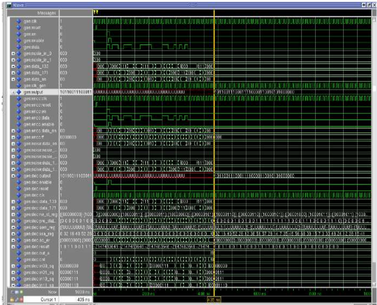
Figure 4.10: Simulation result of 3-bit soft decision viterbi decoder
