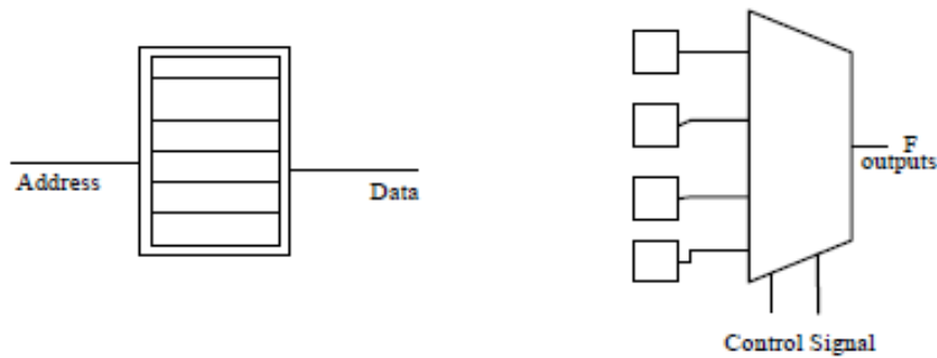
Figure 3.1: Look-up table implemented as (a) Memory (b) Multiplexers and Memory [21]
